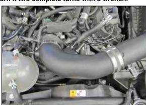
16. Install the K&N® intake tube along with the coupling hose (08536) into the hump hose at the throttle body and then onto the upper air box housing. Secure the hoses with the provided hose clamps.
