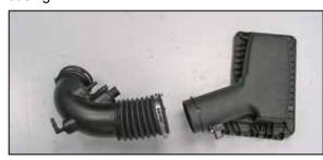
11. Loosen the hose clamp and then remove the factory intake tube from the upper air filter housing
