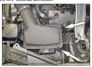
9. Release the two clips securing the air box lid and then remove the lid/intake tube assembly and the factory air filter.
