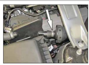
5. Cut the clamp securing the sound tube to the sound drum and then disconnect the sound tube.
