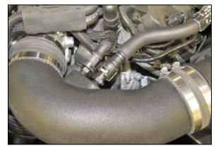
17. Connect the crank case vent and EVAP vent lines to the guick disconnect fittings installed into the K&N® intake tube as shown.
