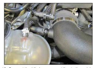
18. Connect the idle by-pass vent line to the quick disconnect fitting installed into the K&N® intake tube as shown.
