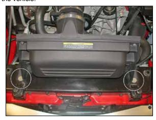
6. Remove the two bolts, which secure the air box to the core support.
