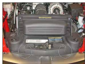
3. Release the center locking pins in the two-core support cover holding clips, and then pull the holding clips out.
