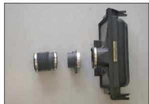
8. Loosen the two hose clamps securing the mass air sensor to the stock air box and intake tube, and then remove the mass air sensor.
