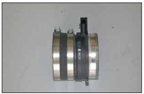
14. Install the provided silicone hose (08536) onto the engine side of the mass air sensor and secure with the provided hose clamp.
