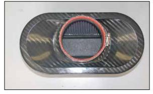
19. Note the flange of the air filter is offset. The offset is to the top of the filter.
