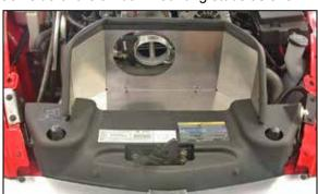
17. Reinstall the core support cover removed in step #5 and secure with the retaining clips removed step #3 and the factory nuts removed in step #4.
