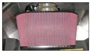
20. Install the air filter onto the mass air sensor and secure with the provided hose clamp.
