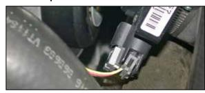
21. Reconnect the mass air sensor electrical connection
