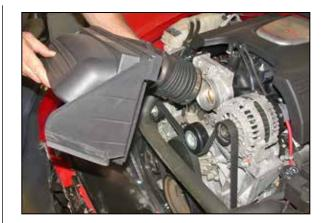
7. Loosen the hose clamp that secures the stock intake tube to the throttle body, and then remove the complete intake assembly from the vehicle. NOTE: K&N Engineering, Inc., recommends that customers do not discard factory air intake.
