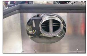
15. Install the mass air sensor assembly onto the K&N® intake tube and secure with the provided hose clamp.
