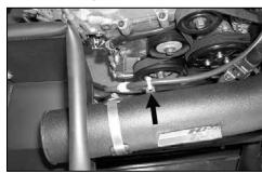
31. Secure the vacuum hose to the K&N<sup>®</sup> intake tube using the provided cable tie.
