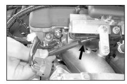
16. On vehicles equipped with air injection pump, attach the air control solenoid valve vacuum hose to the air control valve hard line. (lower hard line).
