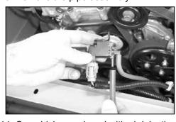
14. On vehicles equipped with air injection pump, attach the provided 4mm (long) vacuum hose to the air control solenoid valve.
