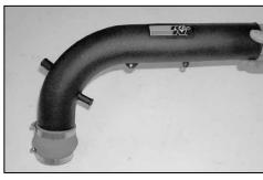
25. Install the silicone hump hose with provided hose clamps, onto the K&N® intake tube as shown.
