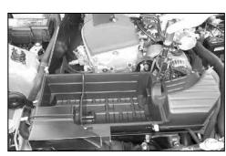
6. On vehicles equipped with air control solenoid, loosen and remove the screw and push clip that secures the air control solenoid valve to the air box base.
