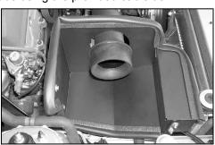
32. Install the radiused adapter onto the K&N $^{\! \rm 8}$  intake tube.
