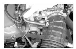
4. Remove the crank case vent hardline from the stock intake tube.
