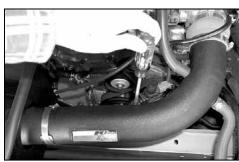
30. On vehicles equipped with an air control solenoid valve, attach the air control solenoid valve to the K&N® intake tube using the original screw removed in step 6.
