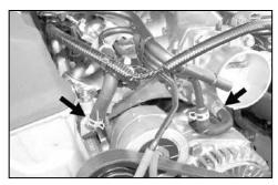
9. Detach the coolant hose from the fitting on the intake manifold, and from the fitting on the underside of the throttle body.
