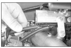
17. On vehicles equipped with air injection pump, attach the check valve vacuum line to the check valve hard line (upper hard line).
