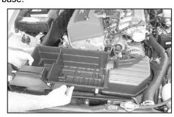
7. Loosen and remove the 3 bolts that secure the air cleaner base, then remove the air cleaner base. NOTE: K&N Engineering, Inc., recommends that customers do not discard factory air intake.
