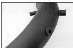
26c. Install the provided grommet into the hole drilled in the  $K\&N^{\mbox{\scriptsize @}}$  intake tube as shown.
