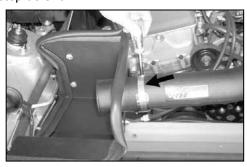
27. Install the K&N<sup>®</sup> intake tube onto the throttle body and align it with the saddle clamp on the heat shield and secure with the provided hose clamps.
