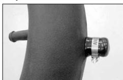
28a. On vehicles not equipped with an air injectino pump, install the provided "Caplug" onto the vent port on the K&N® intake tube and secure with the provided hose clamp as shown.
