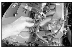
13. Remove the pipe assembly.
