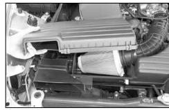
2. Release the 6 clips that retain the air box top, then remove the top.
