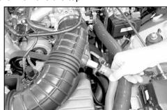
3. On vehicles equipped with air injection pump, detach the air injection pump hose from the stock intake tube.
