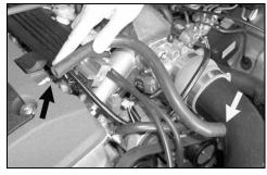
29. Attach the provided 1/2" hose to the crank case vent on the cam cover, then attach the other end to the vent on the K&N® intake tube.
