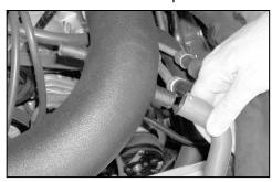
28. On vehicles equipped with air injection pump, attach the air injection hose to the fitting on the K&N® intake tube.
