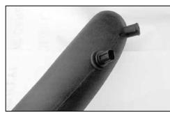
26d. Remove the air temperature sensor from the stock intake tube and install it into the grommet installed in the K&N® intake tube in the provious step as shown.
