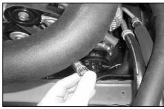
26a. On vehicles equipped with an air temperature sensor, position the air temperature sensor wiring harness on the intake tube for best fit and mark the position on the intake tube with a marker for drilling.
