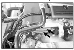
10. Detach the air control valve vacuum hose and the air control solenoid vacuum hose from the hard lines.
