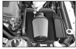
33. Install the K&N® air filter onto the K&N® intake tube and secure with the provided hose clamp. NOTE: Drycharger® air filter wrap; part number RC-5149DK is available to purchase separately. To learn more about Drycharger® filter wraps or look up color availability please visit http://www.knfilters.com®.
