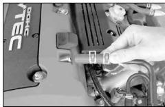
8. Remove the crank case vent hose from the vent on the cam cover.
