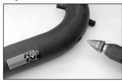
26b. Remove the intake tube from the vehicle and drill a 5/8" id hole in the tube at the position indicated in the previous step.
