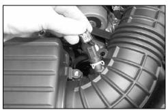
4a. On vehicles equipped with an air temperature sensor, disconnect the air temperature sensor electrical connection as shown.
