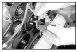
11. On vehicles equipped with air injection pump, detach the vacuum hose from the air control solenoid valve vacuum control solenoid valve.
