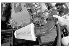
5. Loosen the hose clamp at the throttle body, then, remove the stock intake tube.
