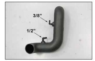
9. Install the two provided 3/8" and ½" 90\* vent fittings into the K&N<sup>®</sup> intake tube as shown. **NOTE: Plastic NPT fittings are easy to cross thread. Install the vent fitting "hand" tight, then turn it two complete turns with a wrench.**
