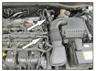
4. Disconnect the EVAP vent hose from intake tube and then disconnect the crank case vent hose from the valve cover. 5. Loosen the hose clamp securing the factory intake tube to the throttle body.
