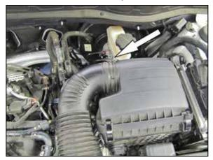
6. Loosen the hose clamp securing the factory intake tube to the air box and then remove the intake tube from the vehicle.
