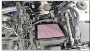
8. Install the provided K&N<sup>®</sup> air filter and then reinstall the upper air box and latch into position.
