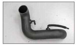
11. Install the 3/8" vent hose assembly onto the 3/8" fitting as shown.
