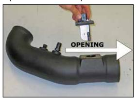
25. Install the mass air sensor assembly into intake tube and secure with the provided hardware.
