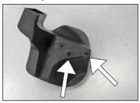
16. Install the airbox mounting grommets onto the two mounting studs installed on the K&N® airbox.
