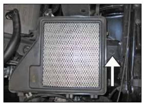
11. Remove the bolt that secures the lower airbox to the inner fender.
