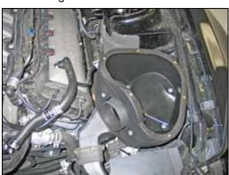
17. Set the K&N® airbox into the vehicle so that the mounting studs slide into the mounting holes, and then secure with the hardware provided.
