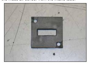
23. Install the provided mass air adapter gasket as shown.
