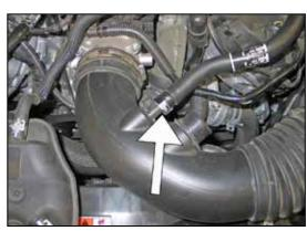
7. Disconnect the crankcase vent hose from the factory intake tube and valve cover port and remove the vent tube from the vehicle.
