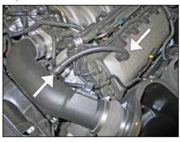
27. Install the crankcase vent hose to the fitting on the K&N<sup>®</sup> intake tube and onto the valve cover. Vehicles equipped with an EVAP vent line, connect it to the fitting installed in the K&N<sup>®</sup> intake tube.
