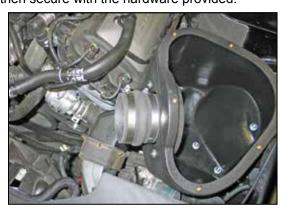
18. Install the provided silicone hose (08418) onto the filter adapter and secure with the provided hose clamp
