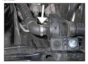
3. Cut the clamp that secures the engine pulse hose to the drum and disconnect the hose from the drum.
