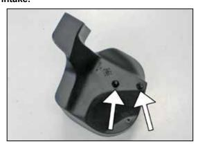
13. Install the two airbox mounting studs onto the bottom of the airbox and secure with the provided hardware.
