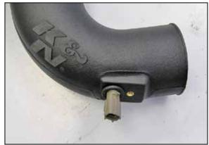
13. Install the temperature sensor into the K&N<sup>®</sup> intake tube and secure with the provided hardware. NOTE: The quarter turn style sensor does not use hardware to hold it in.
