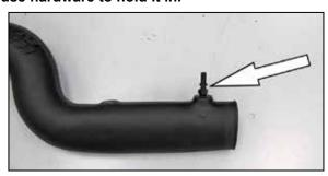
14. Install provided  $\frac{1}{4}$  NPT quick connect fitting onto the K&N® intake tube.
