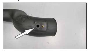
12. Install provided grommet into K&N<sup>®</sup> intake tube
