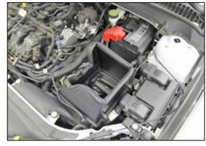
16. Install heat shield onto factory lower air box. Snap in place using factory retaining clips.
