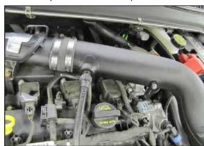
19. Connect crankcase vent line onto quick connect fitting on  $K\&N^{\otimes}$  intake tube.
