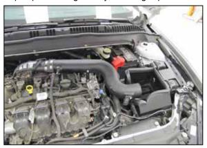
17. Install K&N® intake tube into the hose and onto the tube mounting bracket. Align with heat shield and secure with provided hardware.
