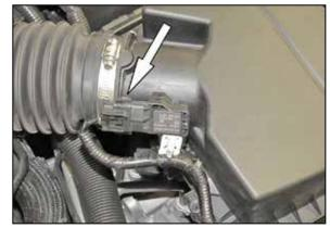
6. Disconnect the temperature sensor electrical connect.
