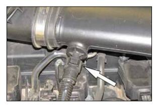
3. Disconnect the crank case vent hose from the factory intake tube by depressing the square locking tab.
