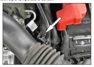
7. Unhook the EVAP tube from the clip on the factory intake tube.
