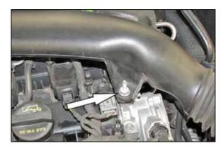
5. Loosen and remove the bolt that secures the intake tube to the engine.
