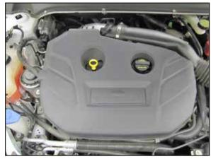
2. Lift up and remove the engine cover from the engine.
