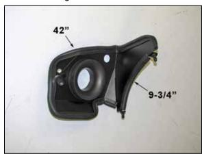
15. Install the provided edge trim onto the heat shield as shown.
