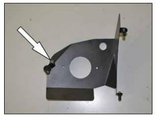
12. Install the bracket assembly onto the heat shield but do not completely tighten at this time.
