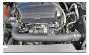
28. Install the K&N® intake tube assembly onto the filter adapter and then onto the throttle body. Adjust the tube and step hose for best fit and then secure with the provided hose clamps.
