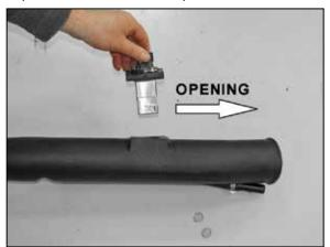
25. Install the mass air sensor into the K&N® tube with the opening facing the direction shown.
