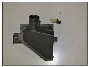
23. Remove the mass air sensor from the air filter housing.
