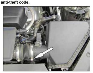
2. Loosen the hose clamp securing the intake tube to the air filter housing.
