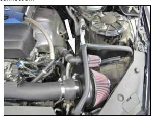
30. On vehicles equipped with secondary air, connect the secondary air hose to the adapter installed into the Heat shield as shown.
