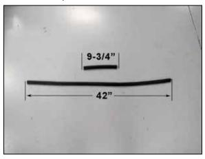
14. Cut the provided edge trim into two sections as shown. One section is 9-3/4" long and the other section is 42"long.
