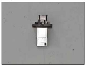
24. Install the mass air sensor into the K&N® adapter and secure with the provided hardware.
