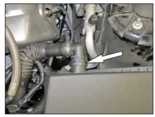
7. Disconnect the secondary air hose from the air filter housing.
