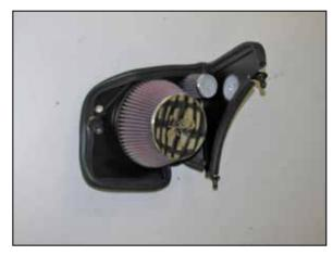
17. Install the K&N® air filter onto the filter adapter and secure with the provided hose clamp.
