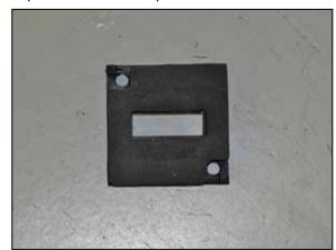
22. Install the provided gasket onto the K&N® mass air adapter.
