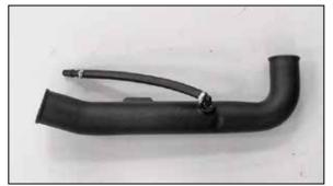
21. Install the vent hose assembly onto the fitting installed into the K&N® intake tube and secure with the provided hose clamp.
