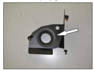
13. Install the filter adapter into the heat shield and secure with the provided hardware.
