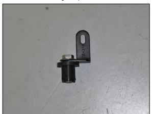
11. Install the insert nut onto the bracket (064319) as shown.
