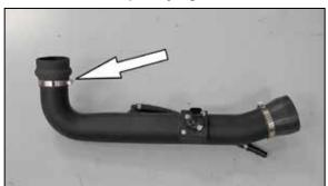
27. Install the provided hump coupler (08185) onto the K&N® intake tube and secure with the provided hose clamp.
