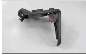
16. Install the secondary air filter onto the heat shield using the provided adapter.
