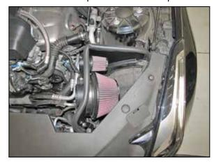
18. Install the heat shield assembly into the engine compartment so the mounting studs go into the mounting grommets and the insert nut goes into the front mounting grommet location. Secure the heat shield by tightening the bolt into the insert nut.
