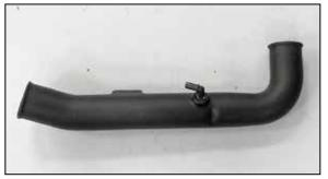
19. Install the provided vent fitting into the  $K\&N^{\otimes}$  intake tube.
