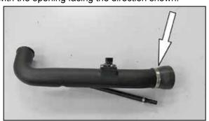
26. Install the provided Step coupler onto the K&N® intake tube as shown.
