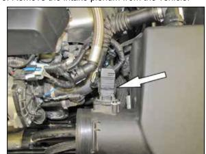
6. Disconnect the mass air sensor electrical connection and unhook the wiring harness from the air filter housing.
