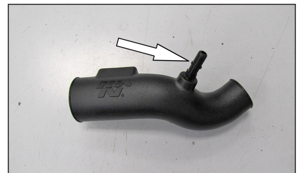
5. Install the provided 1/4" NPT quick disconnect fitting onto the K&N® intake tube. NOTE: Plastic NPT fittings are easy to cross thread. Install the vent fitting "hand" tight, then turn it two complete turns with a wrench.
