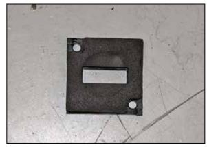
19. Install the gasket on to the K&N $^{\mbox{\tiny B}}$  mass air sensor adapter.
