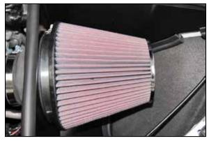
30. Install the K&N $^{\mbox{\tiny B}}$  air filter and secure with the provided hose clamp.
