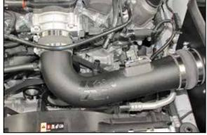
26. Install the K&N<sup>®</sup> intake tube assembly into the coupler at the filter adapter and then into the coupler on the throttle body, adjust the tube for best fit and then secure with the provided hose clamps.
