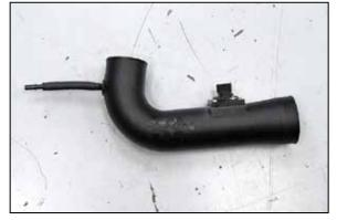
24. Install the EVAP hose assembly onto the K&N<sup>®</sup> intake tube as shown.
