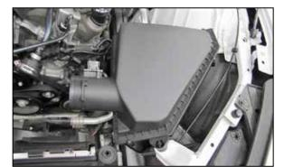
10. Lift up and remove the factory air filter housing assembly.
