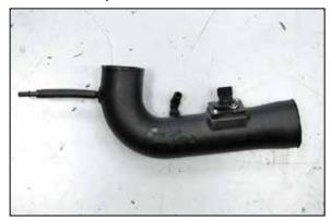
25. Install the 90° crank case vent fitting into the K&N<sup>®</sup> intake tube as shown.
