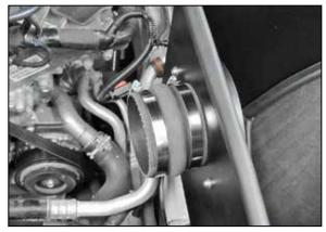
18. Install the provided hump coupler (08699) onto the filter adapter and secure with the provided hose clamp.
