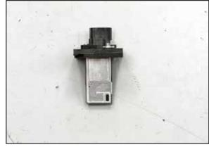
21. Install the mass air sensor into the K&N<sup>®</sup> mass air sensor adapter and secure with the provided hardware.
