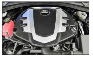
2. Remove the bolt that secures the decorative engine cover, remove the oil cap and then remove the decorative engine cover. Reinstall the oil cap.
