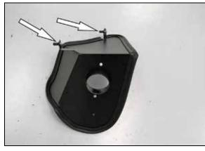
14. Install the two provided mounting posts onto the heat shield using the provided hardware.
