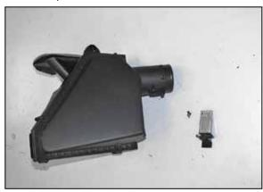
20. Remove the mass air sensor from the factory air filter housing.
