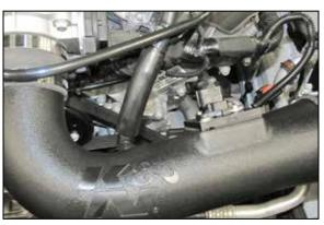
28. Install the provided crank case vent hose onto the factory vent hose and  $K\&N^{\otimes}$  fitting.
