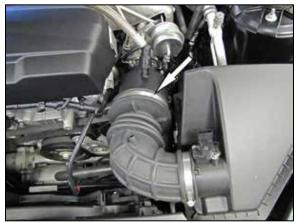
3. Loosen the hose clamp that secures the factory intake tube to the turbo inlet chamber.
