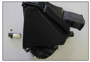
14. Remove the mass air sensor from the factory air filter housing.
