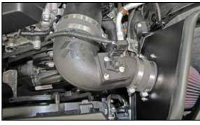
19. Reconnect the mass air sensor electrical connection and secure the wiring harness to the insert in the K&N® intake tube.
