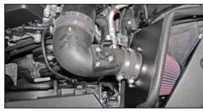
18. Install the K&N® intake tube into the hose at the filter adapter and then into the hose at the turbo chamber, adjust the tube for best fit and then secure with the provided hose clamps.
