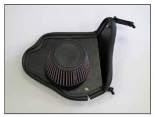
9. Install the K&N  $^{\!0}$  air filter onto the filter adapter and secure with the provided hardware.
