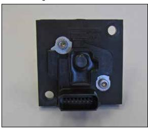
15. Install the mass air sensor into the K&N® mass air sensor adapter and secure with the provided hardware.
