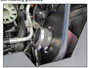
11. Install the provided coupler hose (08711) onto the filter adapter and secure with the provided hose clamp.
