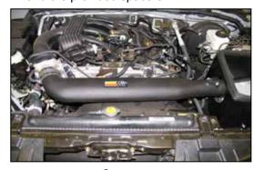
23. Install the K&N® intake tube into the silicone hose at the throttle body and align with the tube mounting bracket installed in step #16. Secure with the provided hardware and hose clamp.
