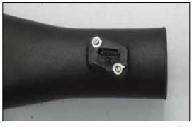
22. Install the mass air sensor into the K&N<sup>®</sup> intake tube and secure with the screws removed in step #21 and the provided spacers.
