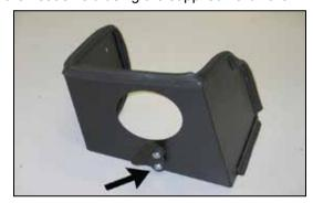
17. Attach the provided "C" bracket (070106) to the rubber mounted studs installed in the previous step using the provided hardware.
