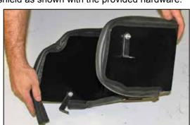
15. Install the edge trim onto the heat shield as shown.
