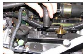
6. Using pliers, loosen the spring clamp which secures the crank case vent hose to the valve cover and then remove the hose from the valve cover as shown.
