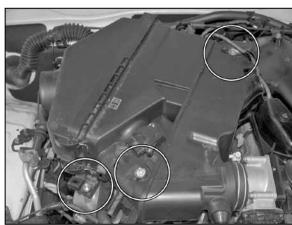
10. Loosen the hose clamp at throttle body, then remove the two bolts that secure air box to engine.
