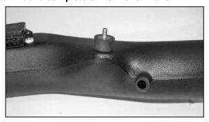
26. Install rubber mounted stud onto K&N® intake tube as shown
