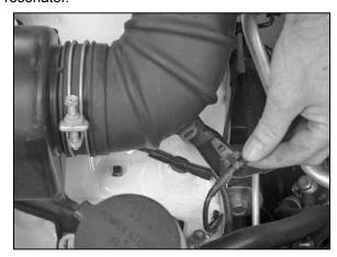
4. Pull wire harness clip up to release from intake tube.
