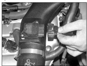
32. Reconnect the mass air sensor electrical connections.
