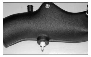
25. Install the vent fitting onto the K&N® intake tube as shown.
