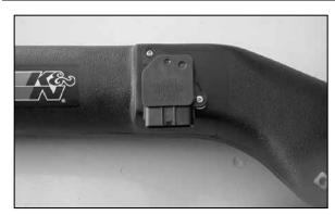
24. Secure the mass air sensor to the K&N® intake tube using the provided screws and spacers as shown.
