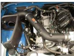
27. Install the K&N® intake tube into the silicone hose at the throttle body and align with the saddle clamp. Secure the intake tube with the provided hose clamps.
