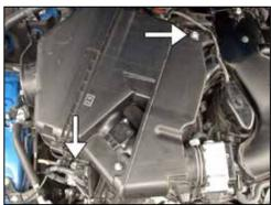
8. Remove the two airbox mounting nuts shown and loosen the hose clamp at the throttle body.
