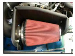
32. Install the K&N® air filter assembly onto the K&N® intake tube and secure with the provided hose clamp.
