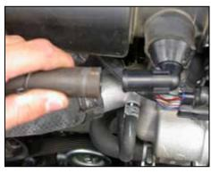
5. Slide the spring clamp back and then disconnect the crankcase ventilation hose from the fitting on the factory airbox.
