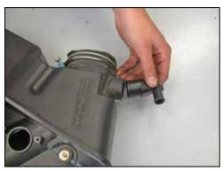
18. Remove the clamp that secures the crankcase vent and then remove the crankcase vent fitting from the airbox.
