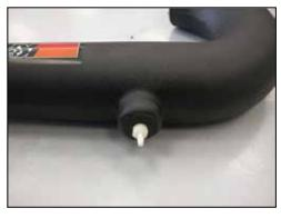
24. Install the supplied ½"npt fitting into the K&N® intake tube as shown.
