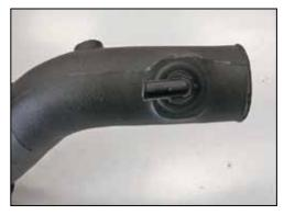
23. Install the stock crankcase vent fitting into the grommet that was installed in the K&N<sup>®</sup> intake tube in the previous step.
