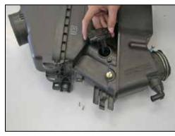
17. Remove the two screws that secure the mass air sensor to the airbox and then remove the mass air sensor from the airbox.
