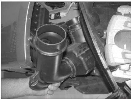
13. Remove the air inlet duct as shown.
