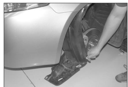
9. Remove the two bolts and three plastic rivets, then, lower the inner fender valance as shown.
