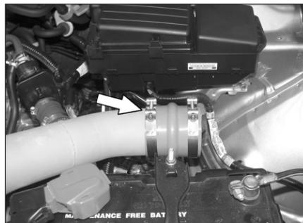
24. Install the silicone hump hose and hose clamps onto the K&N® short ram tube as shown.
