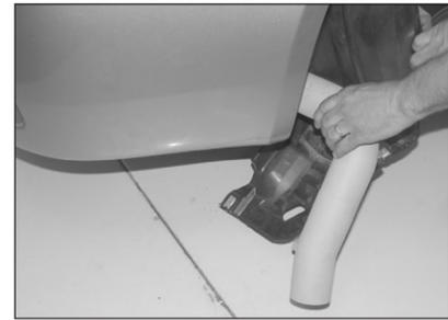
25. Install the cold air tube from underneath the vehicle as shown.
