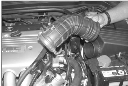
4. Loosen the hose clamp at the throttle body and remove the stock intake tube as shown.
