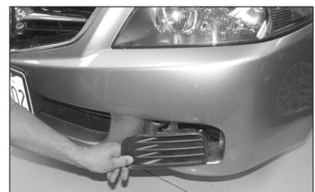
8. Remove the air inlet cover as shown.
