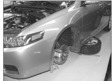
7. Lift the vehicle up and support it with jack stands and remove the front side drivers tire as shown.
