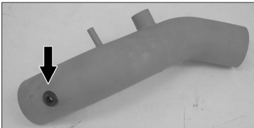
17. Install the provided grommet into the K&N® short ram tube as shown.
