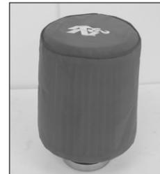
28. Install the K&N® Drycharger® onto the K&N® air filter as shown.
