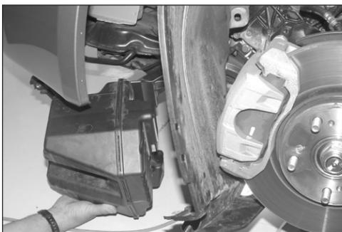
14. Remove the resonator as shown.
