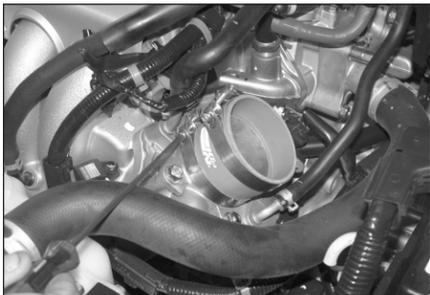
16. Install the silicone hose and hose clamps onto the throttle body and tighten as shown.
