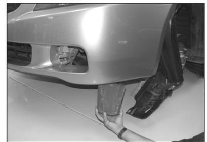
29. Install the filter from underneath the vehicle and secure it using the provided hose clamp.
