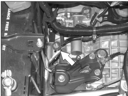
15. Install the rubber mounted stud into the original air cleaner mounting hole as shown.
