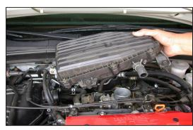
10. Pull firmly upwards to remove the throttle body plenum as shown.
