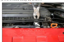
9. Using a pair of pliers, depress and pull back the hose clamp on the crankcase vent at the cam cover.
