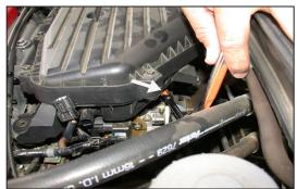
8. Loosen the hose clamp that secures the plenum to the throttle body as shown.
