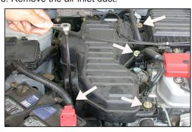
6. Loosen and remove the four bolts that secure the air intake resonator.
