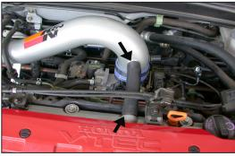
20. Install the provided silicone hose onto the crankcase vent on the cam cover, then connect the other end to the vent on the K&N® intake tube as shown.
