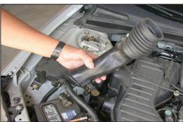
5. Remove the air inlet duct.
