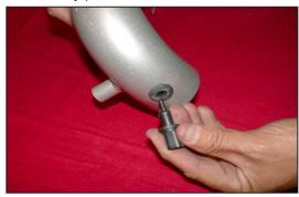
17. Install the provided rubber grommet into the hole on the K&N® intake tube, then install the air temperature sensor into the grommet as shown. NOTE: Before installing the grommet and air temperature sensor, Inspect the inside of the tube for any debris, then clean the inside out with water and a towel. Inspect the tube one more time before proceeding to the next step.
