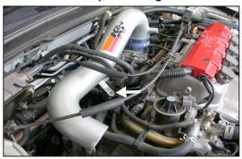
18. Install the K&N® intake tube onto the throttle body, then, line up the bracket with the rubber mounted stud as shown. Tighten hose clamps at this time
