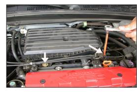
7. Loosen and remove the two bolts that secure the throttle body plenum.
