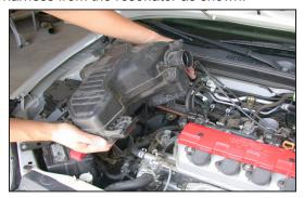
12. Unclip the throttle cable and cruise control cable (If equipped), then, remove the resonator by pulling upwards as shown.
