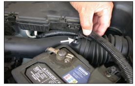
3. Unclip the battery cable from the air inlet duct as shown.
