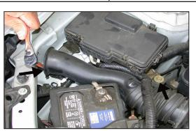
4. Loosen and remove the two bolts that secure the air inlet duct as shown.
