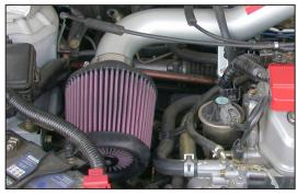
22. Install the K&N® air filter onto the K&N® intake tube and secure with the provided hose clamp. Adjust for best fit and clearance then tighten all hardware.
