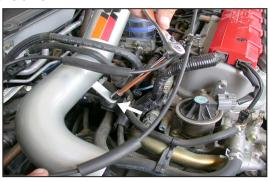
19. Secure the bracket to the rubber mounted stud using the provided hardware, but do not tighten completely at this time.
