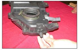
16. Remove the air temperature sensor from the throttle body plenum as shown.
