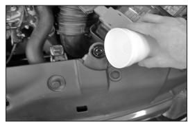
31. Loosen and remove the radiator cap to replace the coolant drained from step #11.
