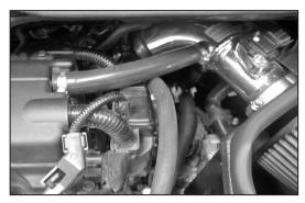
27. Attach the provided CCV-hose with #8 hose clamps, from the engine valve cover to the K&N<sup>®</sup> intake tube as shown.
