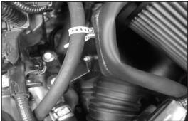
29. Install cable tie to the heat shield, then secure to the hose as shown.
