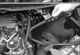
23. Slide the provided hose clamp onto the K&N® intake tube, then install the heat shield. NOTE: On automatic transmission equipped vehicles, it will be necessary to remove the air filter and heat shield from the vehicle to check the transmission fluid level.
