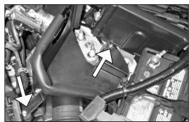
25. Attach the "L" bracket to the heat shield, and then install a bolt through the the hole on the ECU bracket to the threaded boss on the heat shield. Then attach the factory air inlet hose to the heat shield.
