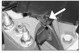
22. Unclip hydraulic line from clip and then remove the clip from the vehicle.
