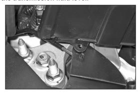
24. Install clip to the hydraulic line then attach to hole in heat shield.
