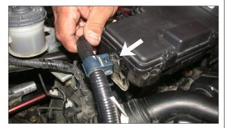
12. Unclip the wire harness from the side of the fuse box as shown.
