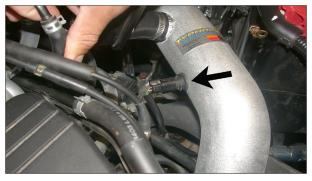
31. Install the air temperature sensor into the grommet on the intake tube as shown.
