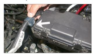
19. Clip the wire harness onto the stock fuse box bracket as shown.
