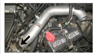
25. Slide the tube into the silicone hose as shown, but do not tighten at this time.
