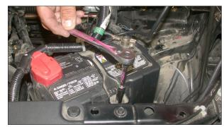
18. Move the battery back into position and secure it with the battery hold down bracket as shown.
