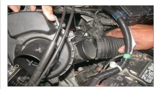
8. Disconnect the air inlet tube from the air cleaner assembly as shown.
