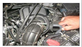
2. Disconnect the vent hose from the stock intake tube as shown.
