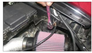
33. Reconnect the ground cable to the inner fender as shown.
