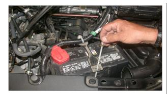
10. Loosen the battery hold down bracket and shift the battery to the left to gain clearance for the removal of the resonator.
