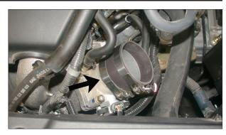
22. Install the silicone hose and hose clamps onto the throttle body and tighten the hose clamp on the throttle body.
