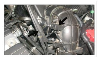
4. Unclip the cruise control cable and the throttle cable from the stock intake tube as shown.
