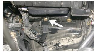
21. Install the provided bracket onto the threaded hole from step 20 and secure with the stock bolt as shown.
