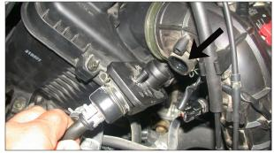
3. Disconnect the crank case vent hose from the stock intake tube as shown.
