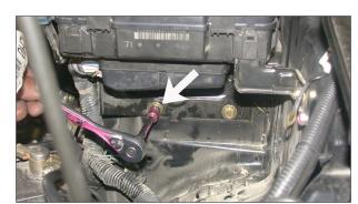
20. Remove the bolt on the lower fuse box bracket as shown.
