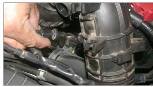
5. Remove the air temperature sensor from the stock intake tube as shown.
