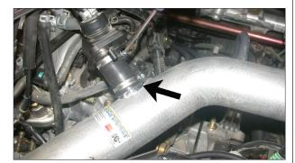
30. Install the provided silicone hose and hose clamps onto the crank case vent, then, connect the other end to the vent on the intake tube as shown.
