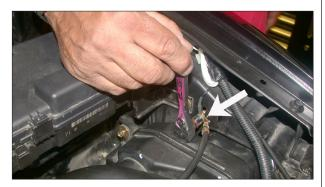
11. Loosen and remove the battery ground at the inner fender as shown.
