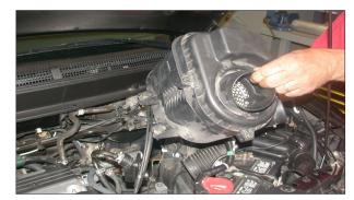
9. Remove the air cleaner assembly as shown. NOTE: K&N Engineering, Inc., recommends that customers do not discard factory air intake.
