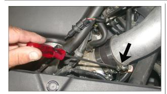
28. Tighten the hose clamp at the throttle body as
