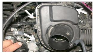
7. Loosen the three bolts that secure the air cleaner assembly to the engine as shown.
