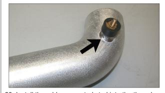
23. Install the rubber mounted stud into the threaded boss on the intake tube as shown.
