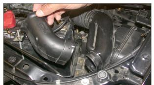
14. Remove the resonator inlet as shown.
