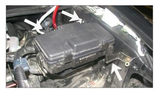
17. Install the fuse box back onto the stock bracket as shown.
