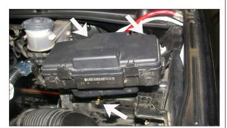
13. Unclip the fuse box (3 places) and lift the fuse box upwards as shown.
