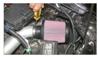
32. Install the K&N air filter onto the intake tube and secure with the provided hose clamp as shown.
