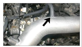
29. Reconnect the vent hose to the vent on the intake tube as shown.
