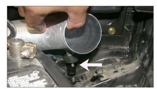
26. Line up the rubber mounted stud with the bracket from step 21 as shown.
