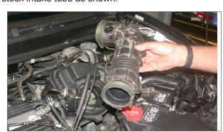
6. Loosen the hose clamps at the throttle body and at the air cleaner, then, remove the stock intake tube as shown.
