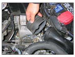
8. Remove the fresh air tube coupler as shown.
