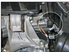
15. Install the provided rubber mounted stud onto the factory air box mounting location as shown.
