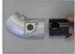
22. Install the venturi into the  $K\&N^{\mbox{\scriptsize 0}}$  intake tube as shown.
