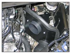
17. Install the heat shield assembly into the vehicle so the mounting grommets attach to the mounting studs, the fresh air tube aligns with the silicone hose, and the silicone hose aligns with the tube in the heat shield. Secure the heat shield with the provided hardware and hose clamp.
