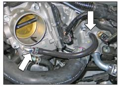
10. Be sure the engine is cool, then disconnect the coolant by-pass hoses from the engine and intake manifold. Install the provided coolant by-pass hose and secure with the factory spring clamps.
