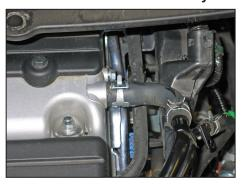
9. Release the spring clamp securing the crank case vent hose to the valve cover and then disconnect the hose from the valve cover.
