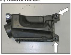
11. Remove the two mounting grommets shown from the factory lower air box.
