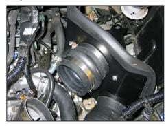
19. Install the provided silicone hose (5-576) onto the filter adapter and secure with the provided hose clamp.
