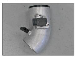
25. Install the mass air sensor into the K&N® intake tube and secure with the provided hardware.
