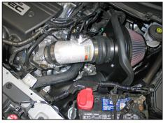
26. Install the K&N® intake tube assembly into the silicone hump hose and then into the throttle body's silicone hose. Align the tube and then secure with the provided hose clamps.
