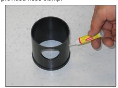
21. Apply several drops of the provided "Super Glue" to the lip of the venturi as shown.
