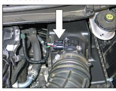
2. Disconnect the mass air sensor electrical connection and unhook the wiring harness from the upper air box.
