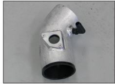
23. Install the provided 90° vent fitting into the  $K\&N^{\oplus}$  intake tube as shown.
