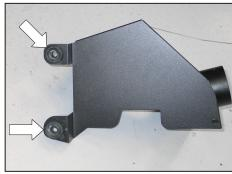
12. Install the mounting grommets from the previous step into the heat shield as shown.
