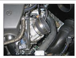
18. Install the provided silicone hose (084034) onto the throttle body and secure with the provided hose clamp.
