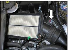
6. Remove the lower air box retaining bolt shown.
