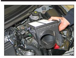
7. Lift up the front of the air box and disconnect the fresh air intake tube, then dislodge the air box from the mounting grommets and remove the air box from the vehicle.
