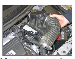
5. Release the two clips securing the upper air box to the lower air box and then remove the upper air box and intake tube assembly.
