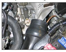
16. Install the provided silicone hose (08637) onto the fresh air intake tube as shown; secure with the provided hose clamp.
