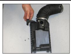
24. Remove the two screws securing the mass air sensor into the factory air box, then remove the sensor from the air box.
