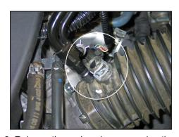
3. Release the spring clamp securing the crank case vent tube into the intake tube and then remove the crank case vent tube from the intake
