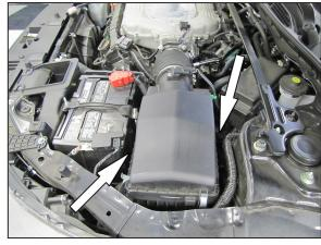
6. Loosen and remove the two air box mounting bolts.
