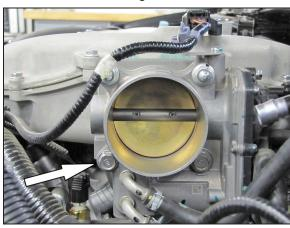
13. Remove the front lower throttle body mounting bolt.
