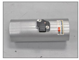
18. Install the mass air sensor into the  $K\&N^{\otimes}$  intake tube and secure with the provided hardware.
