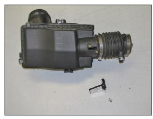
17. Remove the mass air sensor from the factory air box.
