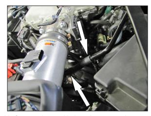
22. Connect the provided crank case vent hose to the factory vent tube and then connect the open end to the 90° vent fitting installed into the K&N® intake tube.
