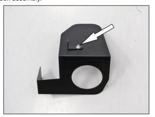
8. Install the heat shield mounting bracket (070015) onto the heat shield as shown.
