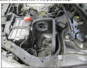
15. Set the heat shield into position on the rubber mounted stud and factory rear air box mounting location. Secure the heat shield with the provided hardware.
