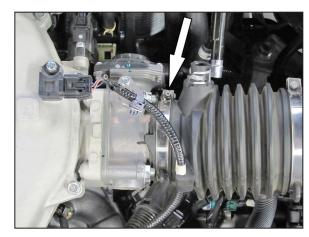
5. Loosen the hose clamp securing the intake hose to the throttle body and unhook the wiring harness from the intake hose.
