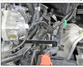
14. Install the provided tube mounting bracket (064302) onto the throttle body and secure with the factory bolt removed in the previous step.
