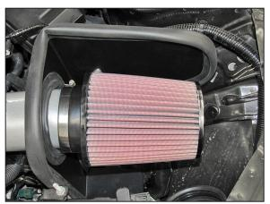
23. Install the K&N® air filter onto the K&N® intake tube and secure with the provided hose clamp. NOTE: Drycharger® air filter wrap; part # RC-4630DK is available to purchase separately. To learn more about Drycharger® filter wraps or look up color availability please visit http://www.knfilters.com®.
