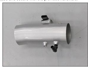
19. Install the 90° vent fitting into the K&N $^{\! \rm 8}$  intake tube as shown.
