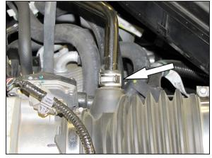
4. Disconnect the crank case vent tube from the intake hose.
