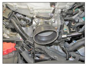
16. Install the appropriate step hose onto the throttle body and secure with the provided hose clamp.
