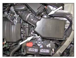
5. Loosen and remove the two bolts securing the factory air box.
