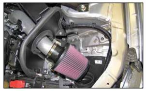
18. Install the K&N<sup>®</sup> air filter onto the K&N<sup>®</sup> intake tube and secure with the provided hose clamp
