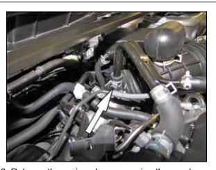
3. Release the spring clamp securing the crank case vent pipe to the factory intake tube and then
