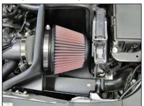
5. Install the K&N<sup>®</sup> air filter onto the filter adapter
