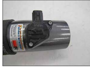
13. Remove the mass air sensor from the factory air filter housing and then install it into the K&N<sup>®</sup> intake tube and secure with the provided hardware.
