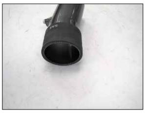
12. Install the provided coupling hose (08711) onto the intake tube so that id slides all the way on. Do not secure the hose now.
