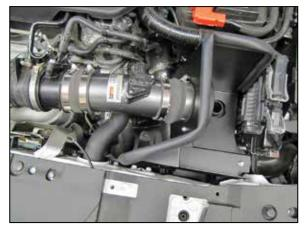
14. Install the K&N<sup>®</sup> intake tube into the coupler at the filter adapter and align with the turbo inlet pipe, slide the coupler back onto the turbo inlet pipe and adjust the tube for best fit. Secure the intake tube with the provided hose clamps.
