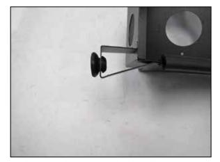
7. Remove the mounting grommet from the factory air filter housing and install it into the K&N<sup>®</sup> heat shield as shown.
