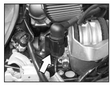
17. Slide the harness multi plug into the bracket as shown.
