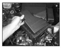
9. Remove the air cleaner assembly from the vehicle as shown.
