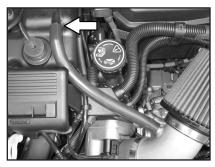
14. Install the provided silicone hose onto the crankcase vent on the cam cover, then, attach the other end onto the vent on the intake tube as shown.
