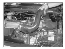
5. Remove the harness multi plug from the side of the air cleaner assembly.
