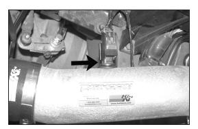
27. Install the air temp. sensor into the rubber grommet on the  $K\&N^{\mbox{\ensuremath{\mathbb{R}}}}$  intake tube.
