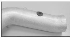
22. Install the smaller grommet into the intake tube.
