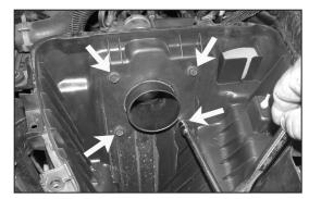
7. Remove the four throttle body retaining bolts from air box. These bolts will be re-used.
