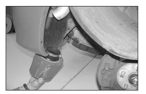
30. From underneath the vehicle, install the K&N $^{\mbox{\scriptsize \$}}$  air filter onto the intake tube.
