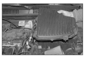
4. Loosen and remove the five air box retaining bolts then remove air box lid as shown.
