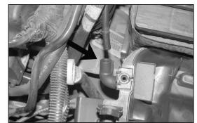
2. Remove the air temperature sensor from the stock intake tube as shown
