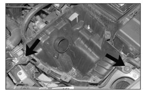
9. Remove the bolt and nut that secure the the air box to the vehicle. Bolt will be re-used.
