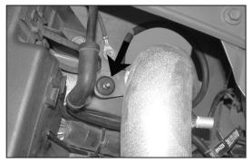
24. Align the intake tube bracket to the stock air box mount.
