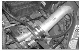
28. Using the supplied silicone hose, attach one end to the K&N<sup>®</sup> intake tube and the other end to the crank case vent tube.
