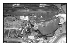
10. Remove the air box from the vehicle. NOTE: K&N Engineering, Inc., recommends that customers do not discard factory air intake.
