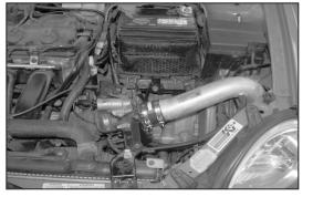
34. Reconnect the vehicle's negative battery cable. Double check to make sure everything is tight and properly positioned before starting the vehicle. 35. The C.A.R.B. exemption sticker, (attached), must be visible under the hood, so the emissions inspector can see it when the vehicle is required to be tested for emissions. California requires testing every two years, other states may vary.
