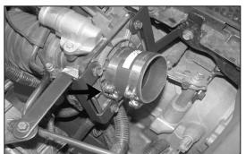
19. Install the supplied silicone hose and hose clamps to the throttle body and tighten throttle body
