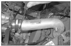
14. Remove the two bolts that retain the resonator to the fender well then remove the resonator.
