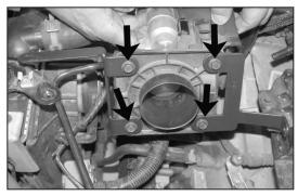
16. Using the four bolts that were removed in step 7, secure the two provided throttle body brackets to the throttle body as shown.
