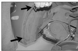
12. Using the supplied T-20 wrench, remove the two screws that retain the inner fender valance to the fender.
