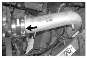
23. Slide the intake tube down the resonator hole then insert the other end into the throttle body silicone hose.
