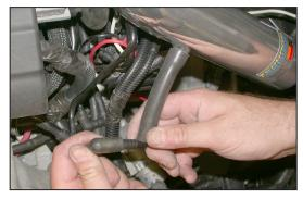
22. Slide the silicone hose onto the vent on the K&N® short ram tube, then connect the 90 degree vent to the stock vent as shown.
