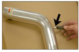
17. Cut a 2" length and a 4-1/2" length of silicone hose from the provided 10" length of silicone hose and install the 2" length hose onto the  $K\&N^{\otimes}$  intake tube as shown.
