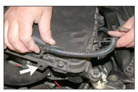
4. Unclip the wire harness from the air cleaner assembly as shown.
