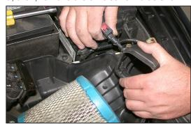
6. Remove the air temperature sensor from the air inlet duct as shown.
