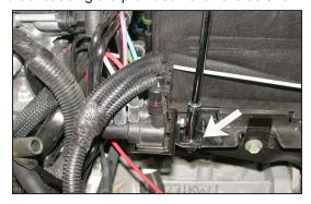
13. Mount the "L" bracket to the battery tray using the bolt removed in step 11.
