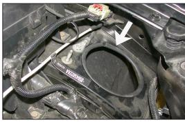
20. Install the provided edge trim onto the hole in the inner fender as shown.
