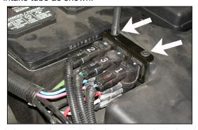
3. Loosen the two bolts that secure the solenoid bracket to the air cleaner assembly as shown.
