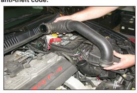
2. Loosen the hose clamp at the turbocharger inlet and at the air cleaner, then, remove the stock intake tube as shown.
