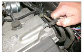
8. Disconnect the crank case vent hose from the cam cover as shown.
