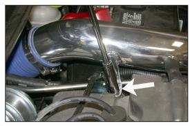
19. Secure the tube bracket to the cam cover stud using the nut removed in step 15 but do not tighten at this time.
