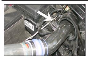
27. Secure the tube bracket to the stud using the nut removed in step 7 and the provided washer, but do not tighten at this time.
