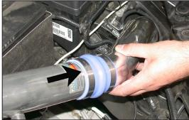
26. Line up the tube bracket with the original air cleaner mounting stud, then, slide the silicone hose onto the short ram tube as shown.
