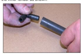
21. Install the 4-1/2" silicone onto the provided 90 degree vent as shown.
