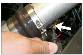
34. Install the air temperature sensor into the cold air tube as shown.
