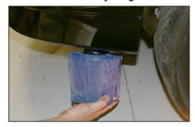
32. From underneath the vehicle install the K&N® air filter and secure with the provided hose clamp.
