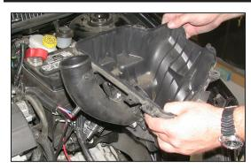
10. Pull firmly upwards to remove the lower air cleaner assembly as shown.
