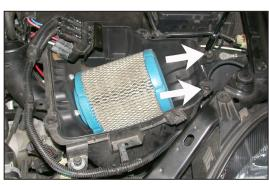
7. Remove the bolt and nut that secure the lower air cleaner assembly to the inner fender as shown.
