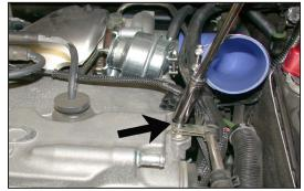
15. Remove the nut that secures the hard line to the cam cover as shown.
