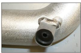
24. Insert the provided rubber grommet into the K&N® cold air tube bracket as shown.
