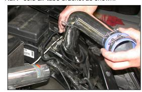
25. Slide the cold air tube into the hole in the inner fender as shown.
