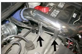
18. Slide the K&N® short ram tube into the silicone hose, then line up the tube bracket with the stud on the cam cover while sliding the silicone hose onto the vent on the cam cover as shown.
