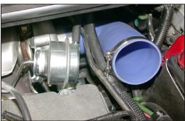
14. Install the silicone hose and hose clamps onto the turbo inlet but do not tighten at this time.
