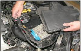
5. Loosen the five bolts that secure the air cleaner lid, then, remove the air cleaner lid as shown.
