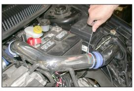
35. Adjust everything for best fit and clearance, then, tighten all hardware and hose clamps as shown.
