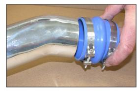
23. Slide the silicone hose and hose clamps onto the K&N® cold air tube as shown but do not tighten at this time.
