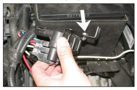
12. Secure the solenoid bracket to the provided "L" bracket using the provided hardware as shown.
