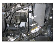
8. Remove the two airbox mounting studs from the frame rail.
