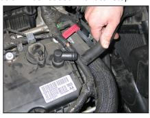
6. Disconnect the crankcase vent hose from valve cover port as shown.
