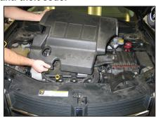
2. Lift up the engine cover and remove it from the engine.
