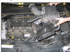
7. Loosen the intake tube hose clamp and disconnect the intake tube from the throttle body. Then lift up and remove the complete stock intake assembly.
