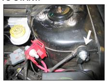
Turn off the ignition and disconnect the negative battery cable at the junction on the strut tower.
