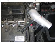
22. Install the provided crankcase vent hose onto the fitting on the valve cover. Then connect the open end to the NPT fitting installed into the K&N® intake tube.
