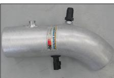
19. Install the inlet air temperature sensor into the grommet installed into the K&N® intake tube.
