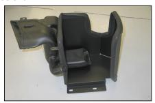
13. Install the fresh air scoop into the heat shield as shown.
