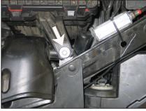
5. Remove the airbox retaining bolt shown. This bolt will be reused in a later step.
