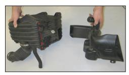
12. Disconnect the fresh air scoop from the airbox as shown.
