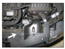
4. Remove the plastic retaining clip which secures the fresh air intake scoop to the core support.
