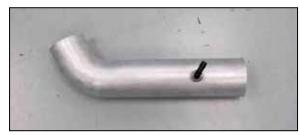
14. Install the 90° vent fitting into the intake tube as shown.
