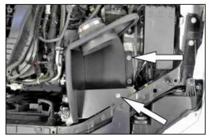
13. Install the heat shield assembly onto the rubber mounted studs and secure with the provided hardware.
