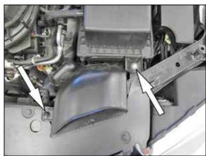
5. Remove the air box retaining bolt and the fresh air intake fastener.
