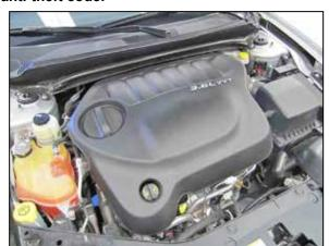
2. Lift up the engine cover and remove it from the top of the engine.
