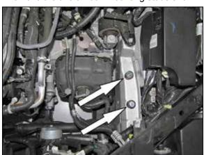
8. Install the two provided rubber mounted studs into the air box mounting stud locations.
