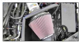
17. Install the K&N® air filter onto the filter adapter and secure with the provided hose clamp. NOTE: Drycharger® air filter wrap; part # RF-1048DK is available to purchase separately. To learn more about Drycharger® filter wraps or look up color availability please visit http://www.knfilters.com®.
