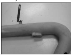
17. Install the supplied "L" bracket and hardware to the K&N® intake kit. Do not tighten completely.
