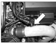
22. Insert the crankase vent line into the rubber grommet on the intake tube as shown.
