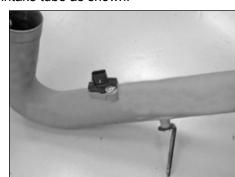
19. Using the stock bolts removed in step # 13, install the mass air sensor into the intake tube as shown.
