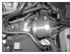
20. Install the supplied silicone hose and hose clamps onto the throttle body and tighten only the hose clamp over the throttle body.
