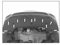
10a. On vehicle's equipped with the splash shield, remove the six bolts and five plastic screws which secure the splash shield to the bumper cover, then remove the splash shield from the vehicle.
