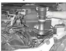
9. Pull firmly up and remove the mass air sensor assembly from the vehicle.
