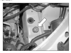
15. Install the supplied rubber mounted stud to the factory threaded hole as shown.
