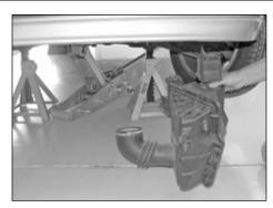
26. On vehicle's that were equipped with an air box cover, reinstall and secure with the bolts that were removed in step #11.
