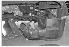
12. On vehicles equipped with an air box cover, lower the cover and remove it from the vehicle.
