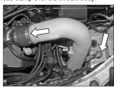
21. Install the intake tube into the vehicle by inserting one end onto the throttle body silicone hose then making sure that the "L" bracket lines up ont the rubber mounted stud.
