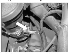
6. Depress the locking tab on the mass air sensor electrical connection and then disconnect the electrical connection.
