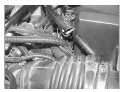
2. Depress the green locking tab on the crank case vent hose and then pull the vent hose to disconnect from the fitting as shown.
