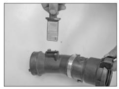
16. Remove the mass air sensor from the stock secondary tube.
