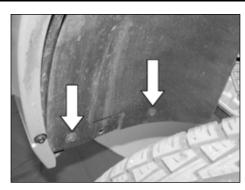
10. After jacking up the car and placing on suitable jack stands and chocking the rear wheels, remove the two bolts which secure the air box on equipped vehicle's or the one bolt on splash shield equipped vehicle's to the inner finder well.
