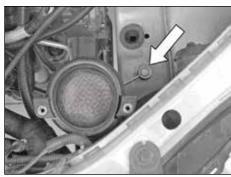
8. Remove the bolt, which secures the mass air sensor housing bracket to the inner fender.
