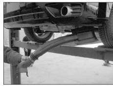
14a. On vehicle's equipped with the upper intake snorkel, pull down on the snorkel to dislodge it from the mount and then remove it from behind the fender.
