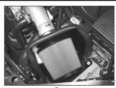
24. Install the K&N<sup>®</sup> air filter onto the intake tube and fasten using the provided hose clamp.
