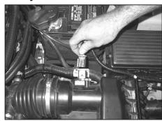
2. Release the red locking clip, then disconnect the mass air sensor electrical connection.
