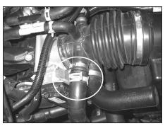
3. On vehicles equipped with an air injection pump, using pliers, release the spring clamp that fastens the air injection hose to the factory intake tube. Disconnect the air injection hose from the intake tube.
