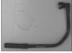
13. Install the supplied silicone vent hose onto the cut end of the stock crank case vent hose.
