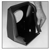
15. Install the provided edge trim onto the heat shield.
