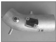
11. Install the mass air sensor into the  $K\&N^{\circledR}$  intake tube using the provided hardware.
