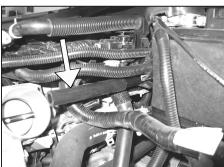
14. Re-install the modified crank case vent hose and fasten using the stock retaining clip.
