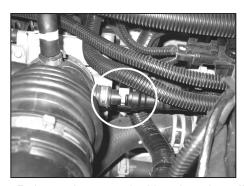
5. Release the green locking ring, then disconnect the crank case vent hose from the stock intake tube.
