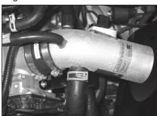
23. Connect the stock air injection hose to the fitting on the  $K\&N^{\circledR}$  intake tube, then fasten using the stock spring clamp.
