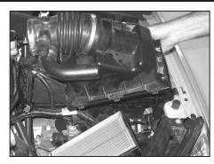
7. Release the three upper air box retaining clips, then remove the upper air box and intake tube assembly.
