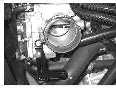
19. Install the intake tube mounting bracket and fasten using the factory bolt removed in step #18.
