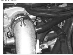
21. Connect the crank case vent hose to the K&N<sup>®</sup> intake tube.
