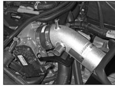
20. Install the K&N $^{\circledR}$  intake tube into the silicone hose (08440) and align the tube mounting bracket (06491) with the intake tube fastening location. Secure the intake tube hose clamps and mounting bracket hardware.
