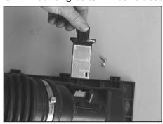
10. Remove the two screws that fasten the mass air sensor to the factory air box, then remove the mass air sensor.
