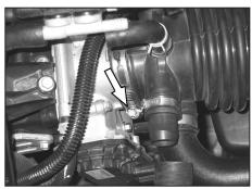
6. Loosen the hose clamp that fastens the stock intake tube to the throttle body.
