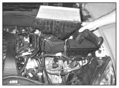
8. Firmly pull the lower air box upwards to dislodge it from the mounting grommets; remove the lower air box.
