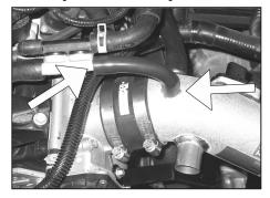
22. Connect the provided silicone solenoid valve hose to the stock fitting and  $K\&N^{\textcircled{R}}$  intake tube fitting.
