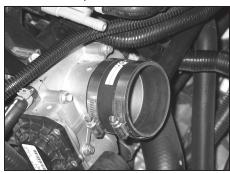
17. Install the provided silicone hose (08440) onto the throttle body and fasten using the provided hose clamp.
