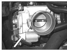
18. Remove the lower throttle body bolt. **NOTE: Bolt will be re-used.**
