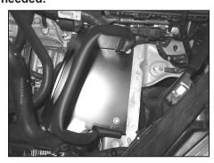
16. Place the heat shield into position in the inner fender well and fasten using the stock bolts removed in step # 9.
