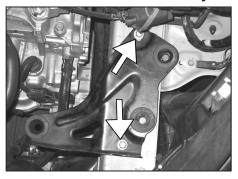
9. Remove the two bolts that fasten the air box mounting bracket to the inner fender, then remove the mounting bracket.
