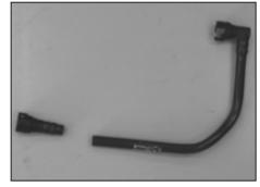
12. Disconnect the crank case vent hose from the valve cover and remove it. Place it on a surface suitable for cutting. Using a a razor blade or knife, cut the crank case vent hose as shown.
