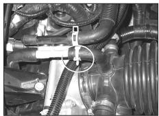
4. Release the spring clamp and then disconnect the solenoid valve hose from the stock plastic fitting
