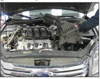
7. Lift up the air box to dislodge it from the mounting grommet and then remove the complete intake assembly.
