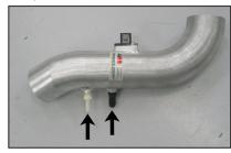
19. Install the two provided  $\frac{1}{4}$  NPT fittings into the  $K\&N^{\otimes}$  intake tube as shown.
