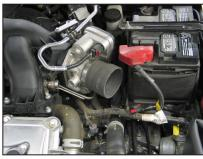
18. Install the silicone hose (08713) onto the throttle body and secure with the provided hose clamp.
