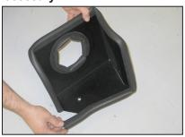
14. Install the long edge trim onto the heat shield as shown.
