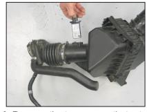
9. Remove the two screws that retain the mass air sensor and then remove the mass air sensor from the air box.
