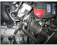
5. Loosen the hose clamp that secures the stock intake tube to the throttle body.
