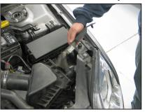
6. Remove the rubber air flap from behind the head light assembly as shown.
