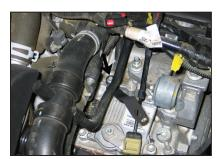
12. Secure the tube mounting bracket to the transmission using the ground strap mounting bolt from step #11.
