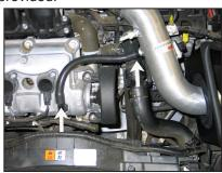
21. Install the provided crank case vent hose onto the valve cover port and then onto the ½"NPT fitting installed into intake tube as shown.
