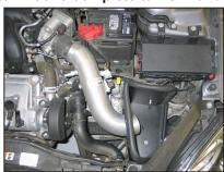
20. Install the K&N® intake tube into the silicone hose at the throttle body and align with the mounting bracket installed in step #12. Secure the intake tube with the hose clamp and hardware provided.
