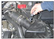
2. Disconnect mass air sensor electrical connection.
