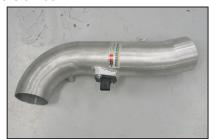
10. Install the mass air sensor into the K&N<sup>®</sup> intake tube and secure with the provided hardware.
