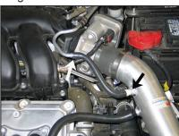
22. On vehicles equipped with an EVAP vent line, install the provided EVAP hose onto the port and then onto the ½"NPT fitting installed into the K&N® intake tube as shown.
