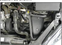
17. Set the heat shield into position on the frame rail and secure with the provide hardware. Secure the rear of the heat shield to the mounting bracket with provided hardware.
