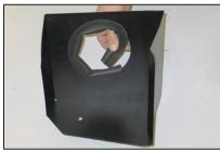
13. Install the short edge trim into the hole of the heat shield as shown.
