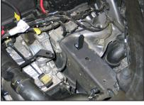
15. Install the heat shield mounting bracket (070602) onto the inner frame rail using the provided hardware as shown.
