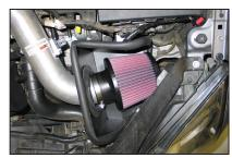
23. Install the  $K\&N^{\otimes}$  air filter and secure with the provided hose clamp.
