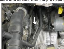
11. Remove the ground strap mounting bolt shown from the transmission.
