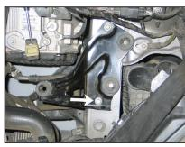
8. Remove the two bolts that secure the air box mount. Then remove the air box mount from the vehicle.
