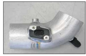
22. Install mass air sensor into K&N® intake tube and secure with the provided hardware as shown.
