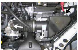
5. Release the three retaining clips securing the airbox lid and loosen the hose clamp at the throttle body.
