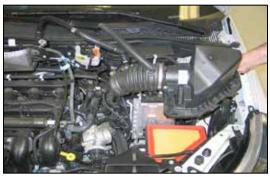
6. Remove factory intake hose and airbox lid from the vehicle.
