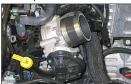
13. Install silicone hose (08440) with provided hose clamps onto the throttle body as shown.
