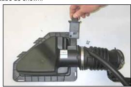
21. Remove mass air sensor from factory airbox lid as shown.
