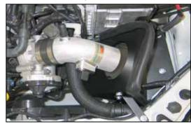
23. Install K&N® intake tube into silicone hose and aligning with tube mounting bracket and heat shield. Secure with provided hardware as shown.
