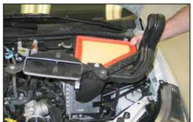
8. Pull up firmly to dislodge the airbox from the grommet and remove the lower airbox assembly from the vehicle as shown.
