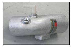
19. Install 90 degree vent fitting into the K&N® intake tube as shown.
