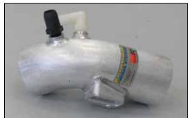
20. Install the 5/8" vent fitting into the K&N® intake tube as shown.
