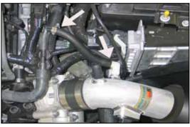
24. Install provided silicone hose onto the EVAP valve with provided hose clamp then onto 90° fitting on K&N® intake tube.
