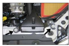
7. Remove the two bolts securing the lower airbox assembly to core support.
