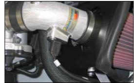
27. Attach mass air extension harness onto factory harness and connect the other end to the mass air sensor electrical connector.
