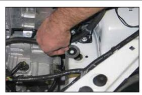
9. Remove airbox grommet from inner fender well as shown.
