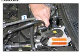
3. Release the locking tab and then disconnect the crankcase vent line from the rear of cam cover as shown
