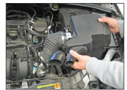
2. Release the red locking tab and then disconnect the mass air sensor electrical connection. Also unhook the mass air sensor wiring harness clip from the mass air sensor.
