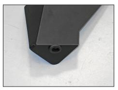
33. Install the provided 7/8"OD grommet into the  $K\&N^{\otimes}$  fresh air plate as shown.
