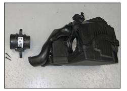
21. Remove the two bolts securing the mass air sensor housing to the air box; separate the mass air housing from the air box.
