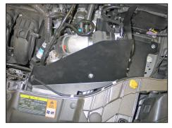
34. Pass the hood release cable through the grommet installed into the K&N<sup>®</sup> fresh air plate and then secure the fresh air plate to the heat shield and mounting bracket with the provided hardware. Reinstall the hood release cable to the hood latch.
