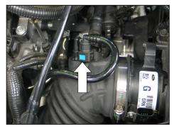
3. Depress the blue locking tab and then disconnect the EVAP vent line.
