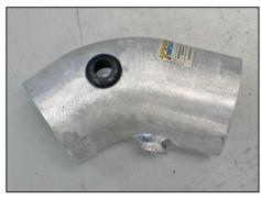
24. Install the provided 1.0"OD grommet into the  $K\&N^{\otimes}$  intake tube as shown.
