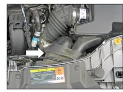
7. Release the rubber strap securing the fresh air intake scoop to the duct.
