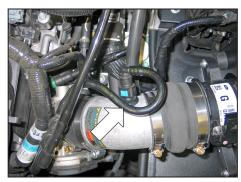
30. Install the EVAP fitting into the intake tube and then connect the EVAP vent line.
