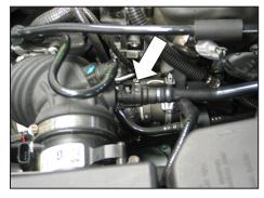
4. Disconnect the crank case vent line from the intake tube.
