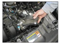
9. Remove the rubber fresh air duct from the vehicle.
