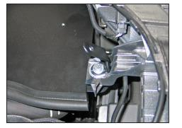
18. Using the provided hardware, secure the provided bracket (083161) to the fresh air intake scoop mount and the rubber mounted stud on the heat shield base.
