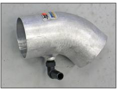
25. Install the 90° vent fitting into the K&N $^{\otimes}$  intake tube as shown.
