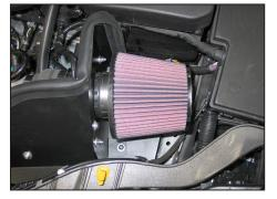
36. Install the K&N<sup>®</sup> air filter and secure with the provided hose clamp.
