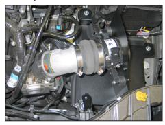
27. Install the K&N<sup>®</sup> intake tube into the silicone hose on the throttle body, then align the heat shield and secure with the provided hardware. Align the intake tube and secure with the provided hose clamps.
