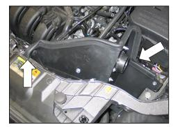
35. Install the 30" long section of edge trim onto the fresh air plate and heat shield as shown. Some trimming of the edge trim will be necessary.
