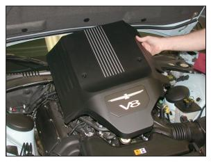
3. Pull up on the rear of the engine cover to dislodge from the retaining mounts, and then remove the engine cover from the engine.
