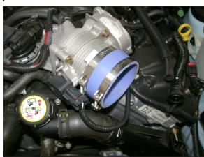
15. Install the provided silicone hose (08698) onto the throttle body and secure with the provided hose clamp.
