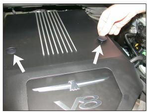
24. Reinstall the engine cover onto the rear retaining clips and then reinstall the retaining clips removed in step #2.
