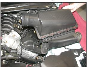
9. Pull up firmly on the air box to dislodge it from the retaining pin, and then remove the air box from the vehicle.
