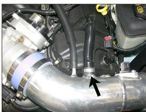
21. Install the large vent hose onto the intake tube as shown.
