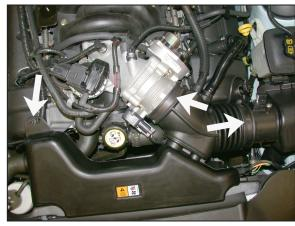
6. Loosen the hose clamps at the throttle body and the factory air box, and then remove the intake tube retaining nut shown.
