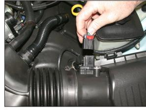
4. Pull back the red locking tab on the mass air sensor electrical connection, and then disconnect the mass air sensor electrical connection.
