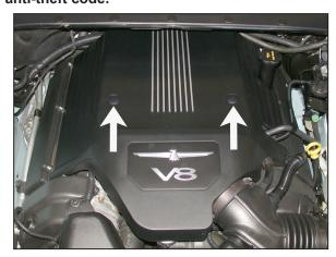
2. Remove the two plastic screws shown securing the engine cover.
