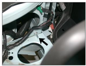
13. Install the provided 6mm bolt through the factory hole in the core support and then install the provided spacer onto the bolt as shown.
