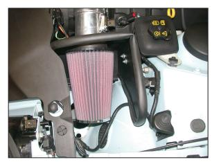
22. Install the air filter and secure with the provided hose clamp.
