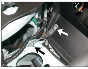
14. Install the provided heat shield bracket (010084) onto the bolt installed in step #14, and then fasten the bracket to the heat shield with the provided hardware.
