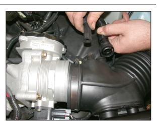
5. Disconnect the hoses from the stock intake tube as shown.
