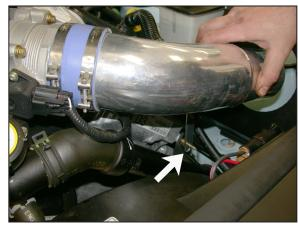
18. Install the intake tube assembly into the silicone hose at the throttle body and slide the bracket onto the stock bolt as shown.
