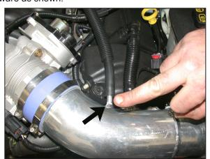
20. Install the small vent hose onto the intake tube as shown.
