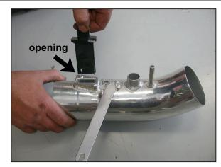
17. Install the mass air assembly into the intake tube and secure with the provided hardware.
