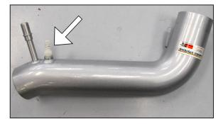
16. Install the provided NPT fitting into the K&N<sup>®</sup> intake tube as shown.
