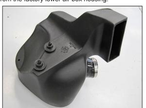
14. Install the air box mounting grommets onto the mounting studs installed onto the K&N® air box during step #10.
