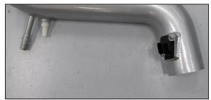
18. Install the mass air sensor into the K&N<sup>®</sup> intake tube and secure with the provided hardware.
