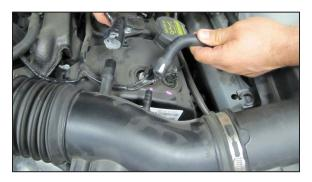
4. Release the locking tab securing the crank case vent hose to the intake tube, then disconnect the crank case vent hose and the EVAP hose from the factory intake tube.
