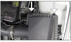
5. Release the two clips that secure the upper air box to the lower air box housing.
