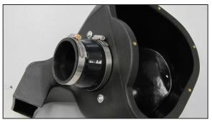
12. Install the provided silicone hose (08724) onto the  $K\&N^{\otimes}$  filter adapter and secure with the provided hose clamp.
