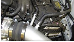
20. Connect the crank case vent hose and EVAP hose to the K&N® intake tube as shown.
