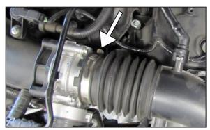
3. Loosen the hose clamp that secures the factory intake tube to the throttle body.
