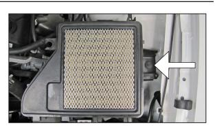
7. Remove the bolt that secures the lower air box to the inner fender shown.
