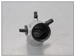
15. Install the venturi into the  $K\&N^{\otimes}$  intake tube as shown.
