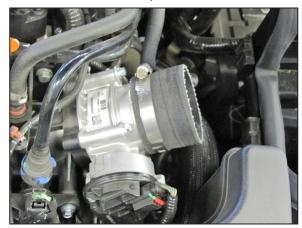
13. Install the provided silicone hose (08440) onto the throttle body and secure with the provided hose clamps.
