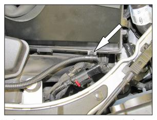
21. Connect the extension harness into the factory harness and then secure the harness to the lower air housing with the mounting tie wrap as shown.
