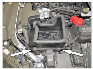
9. Install the heat shield onto the lower air box housing and secure with the factory retaining clips.
