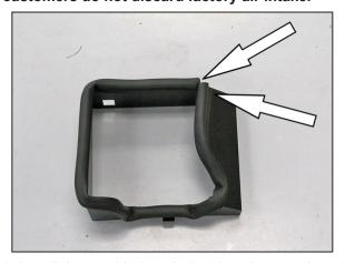
6. Install the provided top bulb edge trim onto the heat shield as shown.
