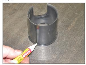
14. Apply several drops of the provided glue to the lip of the venturi insert as shown.
