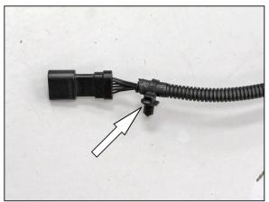
20. Install the provided "Mounting Tie Wrap" onto the female end of the mass air extension harness as shown.
