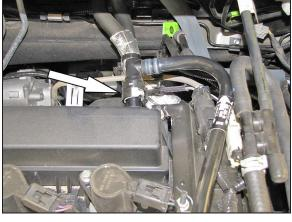
4. Disconnect the crank case vent hose from the valve cover.
