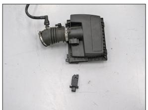
11. Remove the two screws securing the mass air sensor into the upper air box housing and then remove the sensor from the housing.
