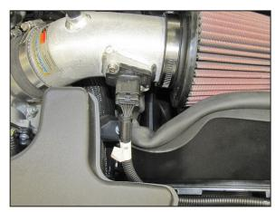
22. Connect the open end of the harness to the mass air sensor as shown.
