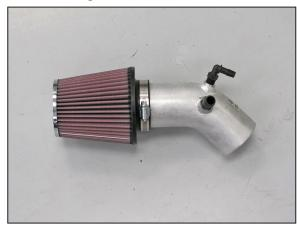
16. Install the  $K\&N^{\otimes}$  air filter onto the  $K\&N^{\otimes}$  intake tube and secure with the provided hose clamp.
