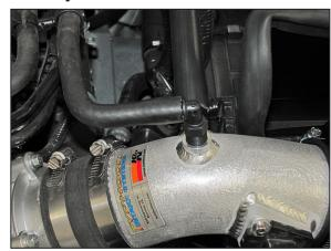
19. Connect the EVAP vent line to the 90° fitting installed into the K&N® intake tube as shown.
