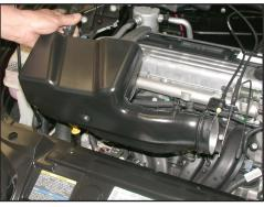
8. Pull upwards to remove the intake plenum as
