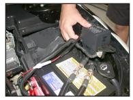
14. Disengage the plastic rivet and pull the fuse box upwards as shown.
