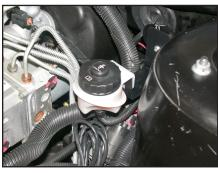
19. On manual transmission vehicles slide the fluid reservoir onto the bracket from step 18 as shown.
