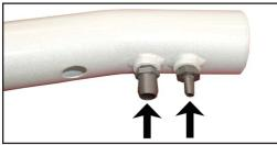
22. Install the two provided 1/4" NPT fittings into the K&N® intake tube as shown.
