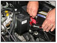
13. Loosen and remove the battery hold down block from the battery tray as shown, and slide the battery forward to create clearance for removal of the lower air cleaner assembly.
