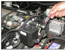
21. Remove the hex nut from the EVAP canister purge solenoid as shown.
