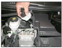
12. On manual transmission vehicles remove the fluid reservoir from the side of the lower air cleaner assembly as shown.
