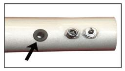
23. Install the provided grommet into the K&N® intake tube as shown.
