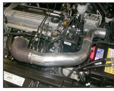
24. Install the K&N® intake tube into the silicone hose at the throttle body and align with the tube mounting bracket installed in step #21a. Secure the intake tube with the provided hose clamp and hardware.
