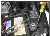
16. Secure the fuse box using the stock plastic rivet as shown.
