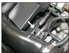
3.Disconnect the vent hose from the stock intake tube as shown.
