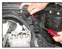
18. On manual transmission vehicles install the provided reservoir bracket onto the air cleaner locater bracket using the provided hardware as shown.
