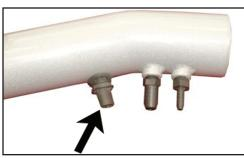
23a. Install the factory inlet air temperature sensor into the grommet installed into the K&N $^{\!0}$  intake tube in the previous step.
