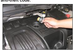
2. Remove the oil filler cap as shown.
