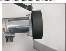
19. With the provided hardware, assemble the filter adaptor and gaskets onto the heat shield and intake tube as shown.
