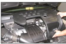
3. Pull firmly upwards to release the engine cover and remove from vehicle.
