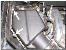
6. Unclip the airbox fastening clips.
