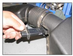
11. Remove mass air sensor from stock intake tube.
