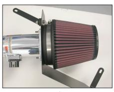
23. Secure the K&N® air filter onto the filter adapter and secure with provided hose clamp.
