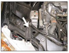
12. Remove the head light mounting bolt and retain as it will be reused.
