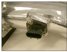
17. Install the mass air sensor onto the K&N® intake tube with provided hardware.
