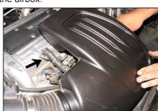
7. Release clamp and remove crankcase vent hose.
