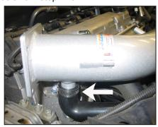
27. On models with air injection, attach the air injection pump hose to the 1" diameter vent fitting on the intake tube and secure with the provided hose clamp.
