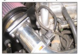
30. Re-connect the mass air sensor electrical connection as shown.
