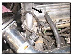
29. Install the silicone hose onto the intake tube vent and onto the crankcase vent line as shown. Tighten hose clamps completely.
