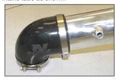
20. Install the silicone hose and hose clamps onto the intake tube as shown.
