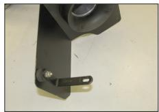
21. Install the rubber mounted stud and small "L" bracket onto the heat shield using supplied hardware. Do not tighten completely at this time.
