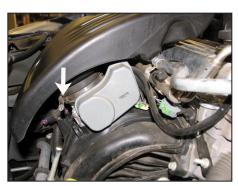
5. Loosen the hose clamp at the throttle body.
