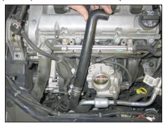
16. On models with air injection, attach the air injection hose assembly to the factory rubber air injection hose and secure with provided hose clamp.
