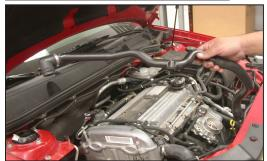
14. On models with air injection, disconnect the air injection pump plastic hard line from the air injection rubber hose.
