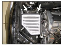
10. Loosen and remove the two airbox retaining nuts then remove the airbox from vehicle.
