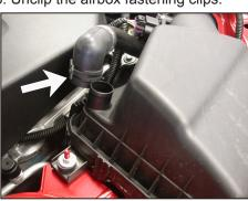
6a. On models with air injection release the clamp and disconnect the air injection pump hose from the airbox.
