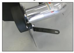
22. Install the rubber mounted stud and "L" bracket onto the heat shield with the provided hardware. Do not tighten completely at this time.
