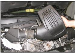
9. Lift firmly upwards and remove airbox from vehicle.
