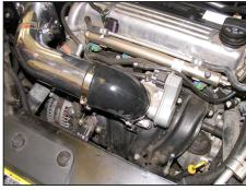
24. Install the intake tube assembly, attaching the silicone hose onto the throttle body as shown.
