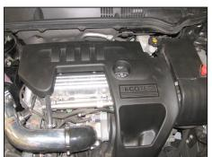
31. Remove oil filler cap so the engine cover can be reinstalled. Reinstall the oil filler cap.
