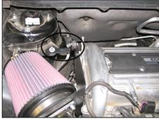
26. Align the heat shield bracket onto the stock airbox mounting stud and secure it with the stock bolt from step #10.
