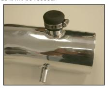
13. On models NOT equipped with air injection, install the provided cap onto the 1" vent fitting and secure with the provided hose clamp.
