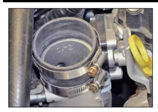
10. Install the provided silicone hose (08476) onto the turbo inlet and secure with the provided hose clamp.
