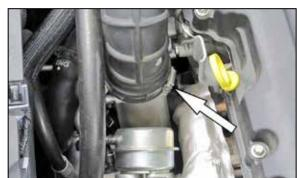
3. Loosen the hose clamp securing the intake tube to the turbo inlet.
