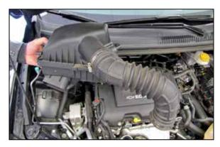
4. Disconnect the intake tube from turbo inlet, and then lift up the air box to dislodge it from the mounting grommets and then remove the air box assembly from the vehicle.
