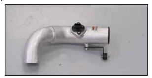
16. Install the tube mounting bracket onto the K&N® intake tube as shown using the provided hardware.
