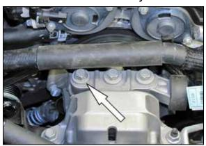
5. Remove the rear engine mount bolt shown. **NOTE: This bolt will be reused.**
