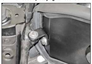
9. Install the provided "L" bracket (070066) onto the core support and heat shield as shown using the provided hardware, then tighten all of the heat shield mounting hardware.
