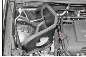
8. Install the heat shield assembly onto the engine mount and secure with the bolt removed in step #5. **NOTE: Do not completely tighten at this time.**
