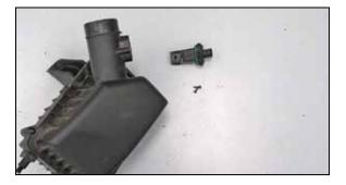
11. Remove the two screws securing the mass air sensor into the factory air box and then remove the mass air sensor from the air.
