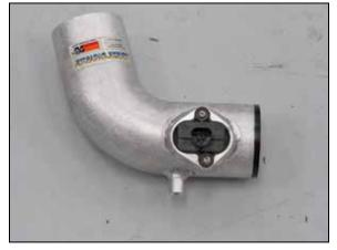
12. Install the mass air sensor into the K&N<sup>®</sup> intake tube and secure with the provided hardware.
