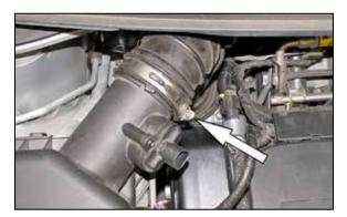
3. Loosen the hose clamp securing the intake hose to the air box and then disconnect the intake hose from the air box.
