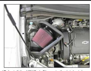
17. Install the K&N® air filter onto the intake tube and secure with the provided hose clamp.
