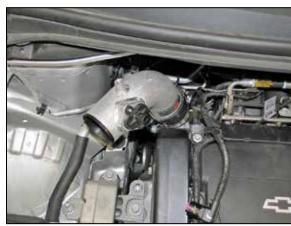
14. Install the K&N® intake tube into the silicone hose but do not completely tighten at this time.
