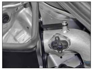
16. Install the tube mounting bracket (010051) onto the heat shield along with the provided spacer. Align the tube and heat shield for proper fit and then secure the bracket, heat shield and intake tube with the provided hardware.
