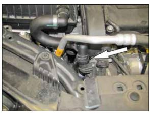
3a. On vehicles that are equipped with air injection, disconnect the air injection hose from the air pump. NOTE: to unlock the air injection fitting, squeeze the outer locking ring to disengage the locking tabs.
