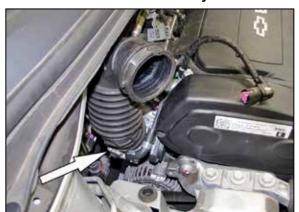
5. Loosen the hose clamp securing the intake hose to the throttle body and then remove the intake tube from the engine.
