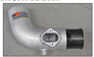
10. Install the venturi into the K&N® intake tube so that the hole lines up with the mass air sensor adapter.
