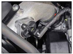
18. Reconnect the mass air sensor electrical connection.
