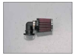
18b. On vehicles equipped with air injection, install the provided breather filter onto the factory fitting from step #11a as shown and secure with the provided hose clamp.
