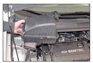
4. Lift up and remove the air box from the vehicle as shown.
