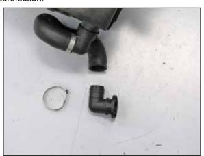
18a. On vehicles equipped with air injection, release the clamp securing the factory air injection fitting to the hose and then remove the fitting from the hose.
