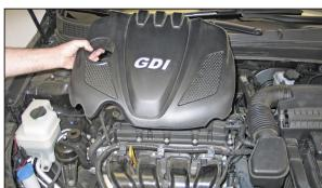
2. Lift up the engine cover to dislodge it from the mounting grommets, remove the engine cover from the vehicle.
