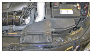
30. Install the fresh air duct and secure with the factory retaining screws.
