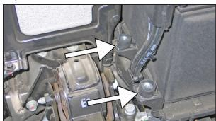
15. Install the two remaining rubber mounted studs onto the airbox mounting locations as shown.
