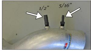
23. Install the two provided vent fittings into the  $K\&N^{@}$  intake tube as shown.
