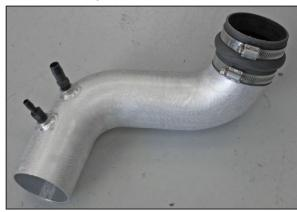
24. Install the provided silicone hose (087121) onto the K&N<sup>®</sup> intake tube and secure with the provided hose clamp.
