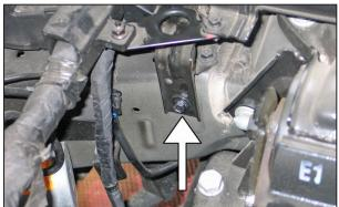
11. Remove the airbox mounting bracket bolt shown.
