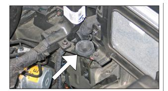
10. Remove the airbox mounting grommet shown.
