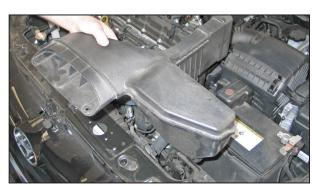
7. Remove the fresh air duct from the vehicle.
