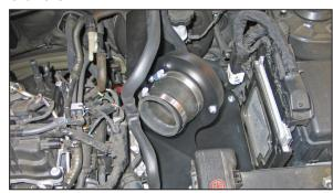
22. Install the provided silicone hose (08724) onto the filter adapter and secure with the provided hose clamps.
