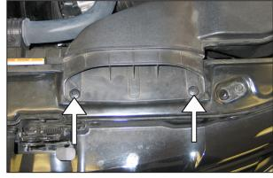
6. Remove the two screws securing the fresh air duct to the core support.
