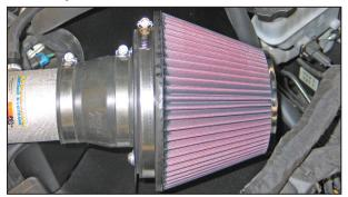
28. Install the K&N® air filter onto the filter adapter and secure with the provided hose clamp. NOTE: Drycharger® air filter wrap; part # 22-8049DK is available to purchase separately. To learn more about Drycharger® filter wraps or look up color availability please visit http://www.knfilters.com®.
