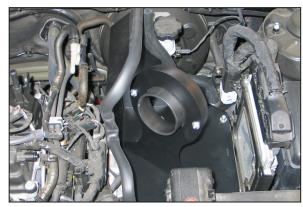
21. Set the heat shield assembly onto the rubber mounted studs and secure with the provided hardware.
