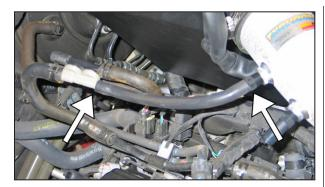
26. On vehicles equipped with an EVAP vent line, Install the provided EVAP hose onto the purge valve and then connect the other end to the vent fitting installed into the intake tube.
