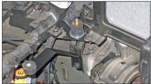
14. Install the provided large rubber mounted stud onto the airbox mounting grommet location using the provided hardware.
