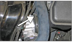
5. Loosen the hose clamp securing the intake tube to the throttle body, then disconnect the intake tube from the throttle body.
