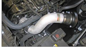
25. Install the K&N® intake tube assembly onto the throttle body and into the silicone hose on the filter adapter, then secure with the provided hose clamps. Tighten the hardware securing the mounting bracket to the heat shield.
