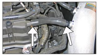
27. Install the provided crankcase vent hose onto the valve cover port and then connect the other end to the vent fitting installed into the intake tube. NOTE: Some trimming of the hose may be necessary.
