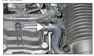
3. Release the spring clamp that secures the crankcase vent hose to the valve cover and the disconnect the crankcase vent hose from the valve cover.
