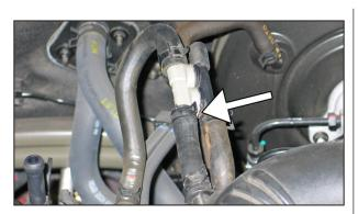
4. On vehicles equipped with an EVAP vent line, disconnect the EVAP hose from the purge valve.
