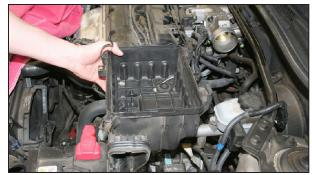
13. Remove the lower airbox as shown. NOTE: K&N Engineering, Inc., recommends that customers do not discard factory air intake.
