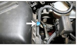
6. Unclip the mass air sensor electrical harness from airbox.
