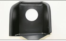
19. Install the provided edge trim onto heat shield as shown.
