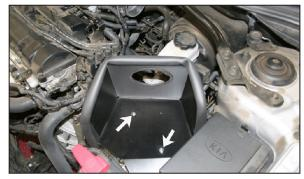
23. Install the heat shield, aligning the rear mounting hole with rubber mounted stud installed in step #21. Align the 2nd mounting hole with the mounting location the fender washers were placed in during step #22. Secure the heat shield in place with the provided hardware.
