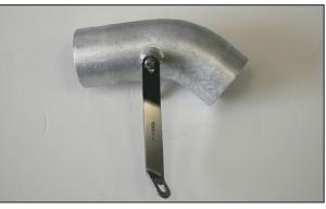
16. Install the provided "C" bracket onto the intake tube and secure it with the provided hardware. **NOTE: Before installing the bracket, inspect** the inside of the tube for any debris, then clean the inside out with water and a towel. Inspect the tube one more time before proceeding to the next step.
