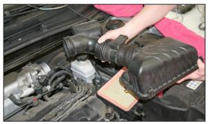
9. Remove the factory intake tube and the airbox lid from the vehicle.
