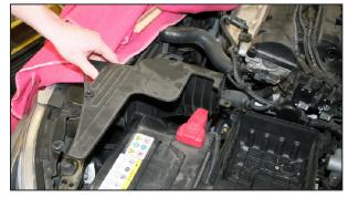
12. Remove the battery cover as shown.
