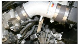
24. Install the intake tube onto the throttle body silicone hose and align the bracket with the bolt hole exposed in step #15. Reinstall the bolt removed in step #15, but do not completely tighten at this time.
