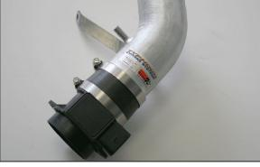
17. Install the mass air sensor onto the the intake tube with the silicone hose and two hose clamps. Tighten the hose clamps at this time.
