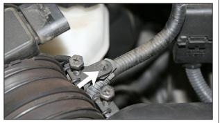
4. Unclip the mass air sensor electrical harness from the factory intake tube.
