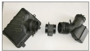
14. Separate the factory mass air flow sensor from the airbox lid and factory tube by loosening the two clamps.
