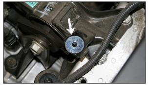
22. Place the rubber washer and fender washer onto the stock airbox mounting hole on the transmission mount as shown.
