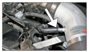
28. Install the crankcase vent hose onto the intake tube.
