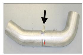
16. Install the provided 1/4npt fitting into the K&N® intake tube as shown.
