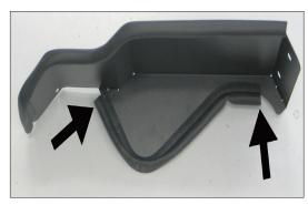
10. Install the 15" long piece of edge trim onto the heat shield as shown.
