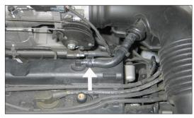
2. Release the spring clamp which secures the crank case vent hose to the valve cover and then unhook the crank case vent hose from valve cover and disconnect the ISC motor wiring harness from the retaining clip attached to the crank case vent hose.
