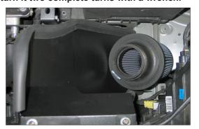
17. Set the K&N<sup>®</sup> air filter into position at the bottom of the heat shield as shown.
