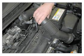
4. Remove the stock intake tube from the vehicle.
