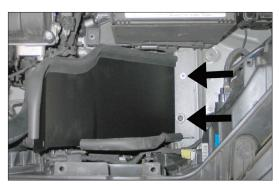
11. Install the heat shield onto the frame rail and secure to the factory stud with the provided hardware and one of the factory air box mounting bolts. **NOTE: Do not completely tighten at this time.**
