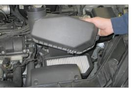
5. Release the upper air box retaining clips and then remove the upper air box from the vehicle.
