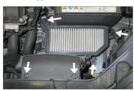
6.Remove the three air box mounting bolts and the two plastic fresh air scoop retaining screws shown.
