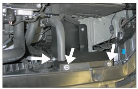
12. Secure the K&N® fresh air scoop to the core support and heat shield using the provided hardware.
