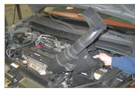
7.Remove the lower air box housing from the vehicle.
