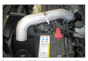
18. Install the K&N® intake tube into the silicone hose at the throttle body and align with the tube mounting bracket. Secure the intake tube with the hose clamp and hardware provided.
