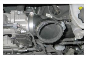
15. Install the provided silicone hose (084087) onto the throttle body and secure with the provided hose clamp.
