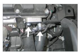
14. Install the K&N® tube mounting bracket (083134) onto the cylinder head and secure with the provided hardware.
