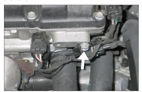
13. Remove the wiring harness retaining bracket bolt shown.
