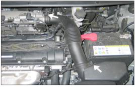
3. Loosen the hose clamps which secure the stock intake tube to the throttle body and air filter housing.
