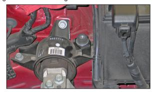
15. Using the provided fender washers, secure the ½" rubber mounted stud to the airbox mounting bracket as shown.
