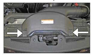
6. Remove the two bolts securing the fresh air intake duct to the core support and then remove the fresh air duct from the airbox.
