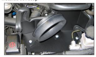
24. Install the bracket/filter adapter assembly onto the heat shield and secure with the provided hardware.
