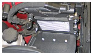
21. Secure the ECU assembly to the heat shield as shown using the provided hardware.
