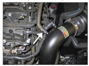
30. On vehicles equipped with an EVAP vent line, attach the factory vent line to the straight vent fitting installed into the K&N® intake tube.
