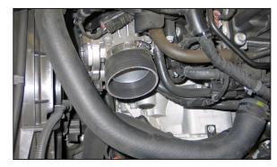
22. Install the silicone hose (084036) onto the throttle body and secure with the provided hose clamp.
