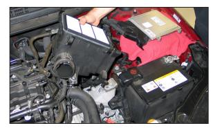
10. Separate the ECU from the airbox and set aside, then remove the airbox from the vehicle.
