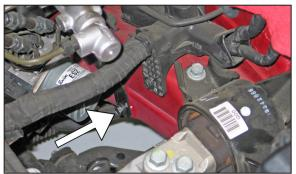
12. Remove the specified bolt securing the ABS pump bracket to the inner fender.
