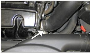
5. Loosen the hose clamp that secures the factory intake tube to the throttle body.
