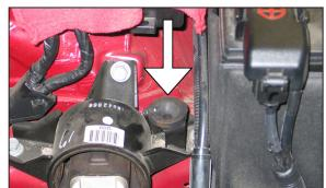
14. Remove the specified airbox mounting grommet from the engine mount bracket.
