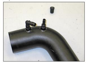
26. Install the two vent fittings into the  $K\&N^{\text{\scriptsize \$}}$  intake tube as shown.
