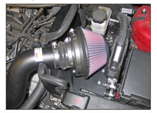
28. Install the K&N® air filter onto the filter adapter and secure with the provided hose clamp.
