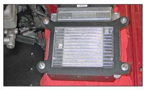
20. Secure the ECU to the rubber mounted studs with provided hardware.
