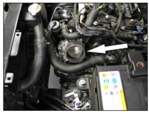
13. Install the provided hump hose (08421) onto the throttle body and secure with the provided hose clamp.
