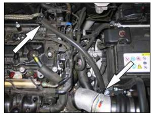
20. Install the provided crank case vent hose onto the 90° vent fitting and valve cover port as shown.
