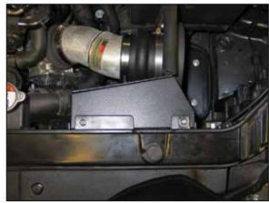
21. Install the K&N® fresh air intake scoop and secure to the heat shield and core support with the provided hardware.
