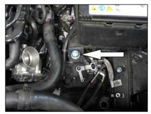
12. Install the  $\frac{1}{2}$ " rubber mounted stud onto the air box mounting grommet location using the provided fender washers on both sides of the mounting bracket.
