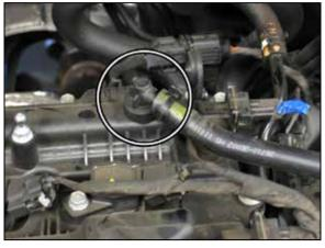
3. Release the spring clamp securing the crank case vent hose to the valve cover port and then disconnect the crank case vent hose from the valve cover.
