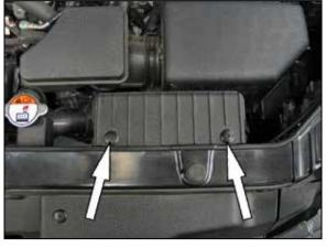
4. Remove the two plastic screws securing the fresh air intake scoop and then remove the clips.
