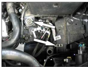
10. Remove the air box mounting grommet shown, and then remove the inner most ground strap bolt shown.
