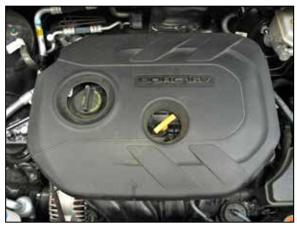
2. Pull up the engine cover and remove it from the engine.
