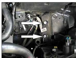
11. Install the two 1" rubber mounted studs as shown. One will screw into the threaded hole vacated by the ground strap bolt in step #10 and the other will thread onto the unoccupied stud on the frame rail.
