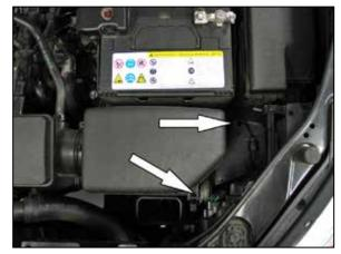
7. Unlatch the two upper air box retaining clips.
