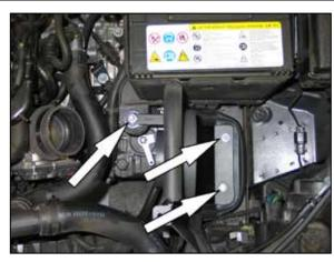
17. Install the heat shield onto the rubber mounted studs and secure with the provided hardware.
