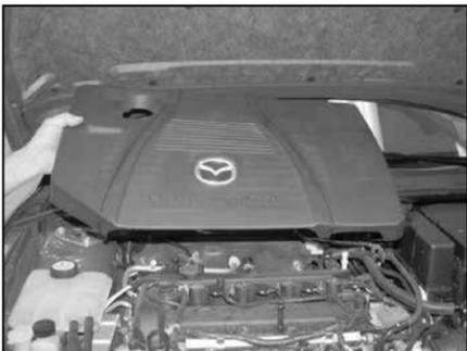
2. Unclip the battery cover and remove, then, disconnect the negative battery cable.
