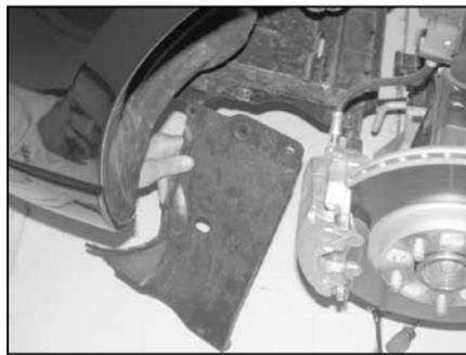
20. Remove the four bolts and one plastic rivet from the inner valance then, remove the valance as shown.
