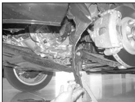
21. Remove the three plastic rivets and six hex bolts on the inner wheelhouse valance, then, pull the inner wheel house valance downward as shown.
