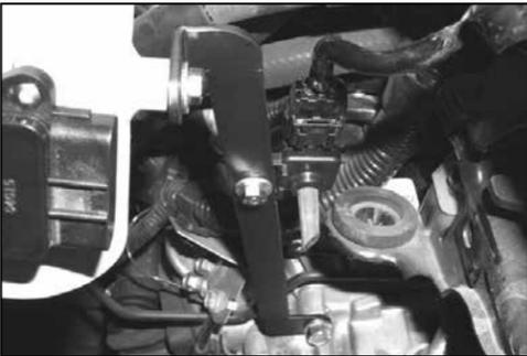
28. Secure the switch from step 7 to the bracket using the provided hardware as shown.
