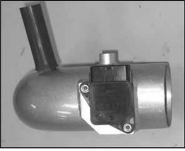
26. Install the mass air sensor into the intake tube using the provided hardware as shown.
