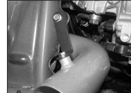
36. Secure the bracket to the rubber mounted stud using the provided hardware as shown.
