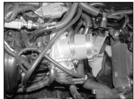
24. Install the silicone hose and hose clamps onto the throttle body as shown.
