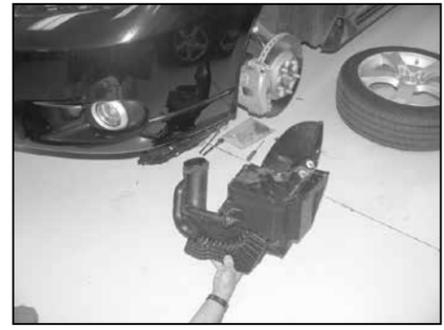
22. Remove the three bolts that secure the air intake resonator to the inner fender, then, remove the resonator as shown.
