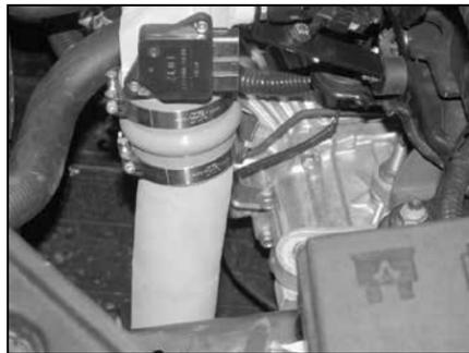
35. Slide the cold air tube onto the short ram tube as shown.
