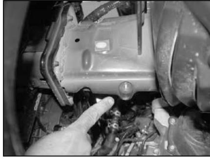
31. Install the provided rubber mounted stud into the resonator threaded hole as shown.
