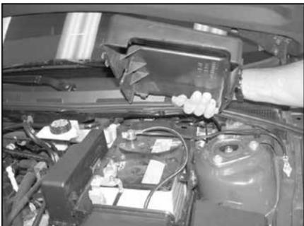
3. Disengage the plastic rivet as shown.
