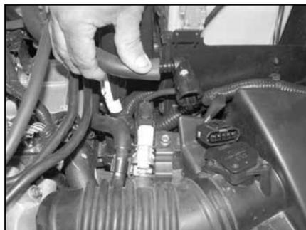
6. On vehicles equipped with a quick release crankcase vent hose fitting, release the fitting and disconnect the crankcase vent hose from the intake tube. On vehicles not equipped with a quick disconnect fitting, unplug the crankcase vent fitting from the intake tube.
