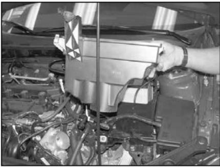
12. Remove the lower air cleaner assembly as shown.
