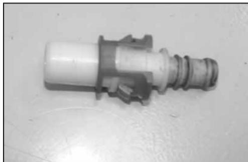
18. On vehicles equipped with the crankcase quick disconnect fitting, slide the plastic clip from step 15 back onto the crankcase vent as shown.
