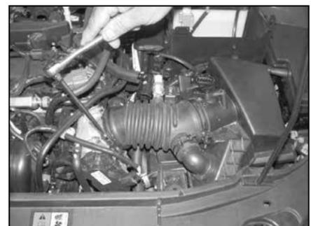
8. Loosen the hose clamp at the throttle body as shown.
