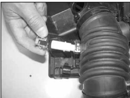
15. On vehicles equipped with the crankcase quick disconnect fitting, remove the plastic clip from the crankcase vent on the stock intake tube as shown.
