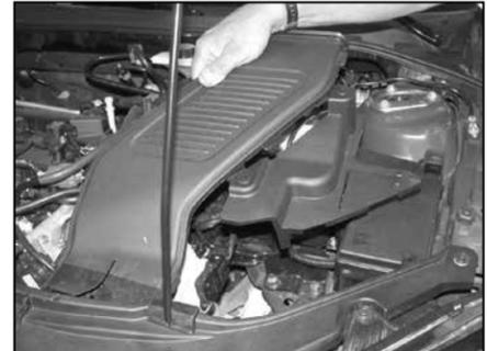
42. Slide the vent into the core support and line up the other end with the battery box and secure with plastic rivet.
