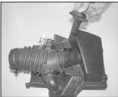
14. Remove the mass air sensor from the air cleaner cover as shown.
