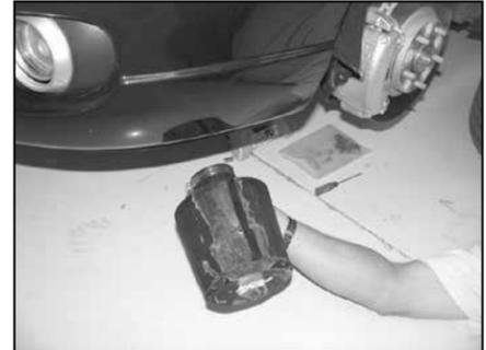
38. Install the air filter onto the cold air tube from underneath the vehicle as shown.
