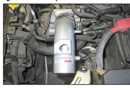
20. Slide the K&N® short ram tube into the silicone hose, then line up the "L" bracket with the rubber mounted stud and secure with the provided hardware as shown.
