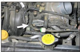
16. Disconnect the airbox vacuum hose shown from the intake manifold, and then plug the intake vacuum port with the provided vacuum plug.
