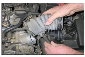
6. Loosen the hose clamps at the throttle body and at the mass air sensor, then pull the stock intake tube up and unclip the hoses from the bottom of the intake tube as shown.
