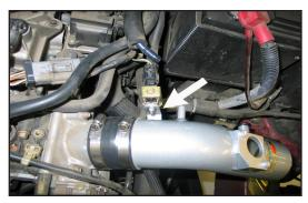
21. Secure the vacuum switch from step 7 to the intake tube bracket using the existing hex nut from step 7.
