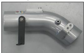
19. Install the "L" bracket onto K&N® intake tube with hardware provided as shown.
