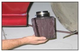
32. Install the K&N® Drycharger® onto the K&N® air filter; from underneath the vehicle install the air filter onto the cold air tube and secure with the provided hose clamp as shown.
