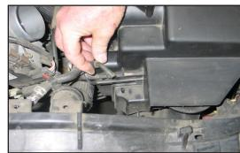
8. Disconnect the vacuum hose from the air cleaner as shown.
