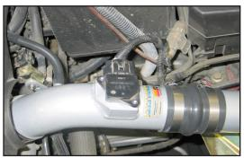
35. Reconnect the mass air sensor electrical connection as shown.
