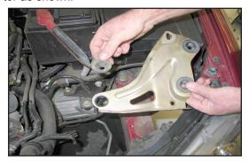
13. Loosen and remove the two bolts that secure the air cleaner support bracket to the inner fender, then remove the stock rubber grommet as shown.
