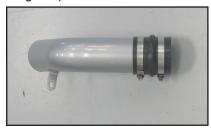
29. Slide the silicone hump hose and hose clamps onto the intake tube as shown.
