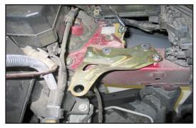
15. Using the provided hardware reinstall the air cleaner support bracket back into the vehicle turning it upside down as shown.
