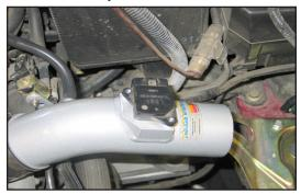
28. Install the mass air sensor into the intake tube using the provided hardware as shown.
