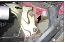
24. Remove the bolt that secures the ground block to the inner fender as shown.
