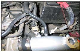
22. Connect the provided silicone hose to the crankcase vent hard line, then connect the other end to the vent on the intake tube as shown.
