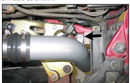
31. Line up the bracket on the cold air tube with the rubber mounted stud; secure with the provided hardware as shown.
