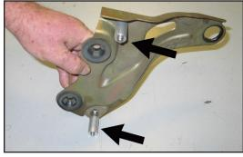
14. Install the provided spacers, washers and hex bolts into the holes on the stock support bracket as shown.
