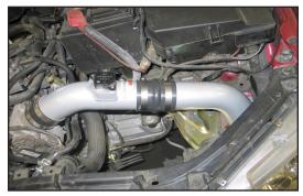
30. Install the intake tube into the hole in the inner fender, then slide the hump hose onto the short ram tube as shown.
