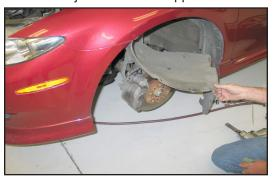
11. Remove the 4 screws and 5 plastic rivets from the inner fender valance, then pull the valance back as shown.
