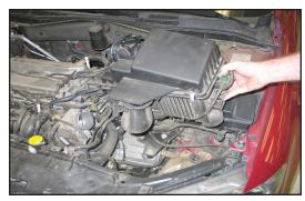
9. Unclip the mass air sensor electrical connection from the side of the air cleaner, then, pull firmly upwards to release the air cleaner from the factory grommets as shown.
