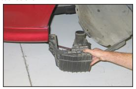
12. From underneath the vehicle, loosen and remove the 3 bolts that secure the air intake resonator to the inner fender, then remove the resonator as shown.
