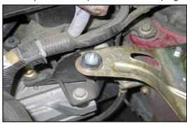
17. Using the provided fender washers and rubber washer, secure the provided rubber mounted stud onto the air cleaner support bracket as shown.
