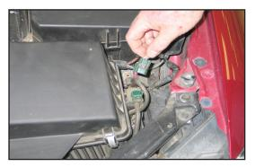
4. Disconnect the vacuum switch electrical connection as shown.
