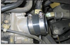
18. Install the silicone hose and hose clamps onto the throttle body as shown.
