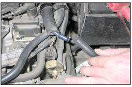
5. Disconnect the crankcase vent hose from the hard line as shown.
