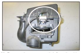
23. Remove the vacuum switch from the side of the air cleaner assembly as shown.
