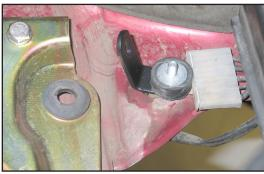
25. Install the angle bracket and rubber mounted stud into the threaded hole from step 24.
