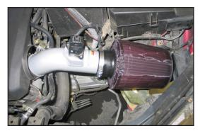
37. This K&N® high flow intake system has been designed to be used in two different configurations. In the case of inclement weather, the cold air tube can be removed and the air filter can be clamped onto the intake tube located in the engine compartment to avoid the possibility of ingesting water into the engine.
