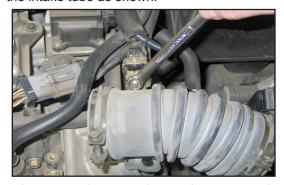
7. Loosen and remove the nut that secures the vacuum switch to the stock intake tube as shown, then remove the stock intake tube.
