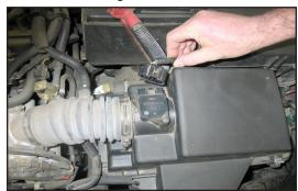
3. Disconnect the mass air sensor electrical connection as shown.
