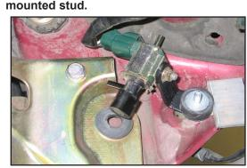
26. Install the vacuum switch from step 23 onto the angle bracket using the stock nut from step 23; then reconnect the vacuum switch electricalconnection.
