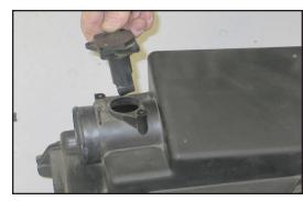
27. Remove the mass air sensor from the stock air cleaner assembly as shown.
