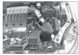
32. Install the K&N<sup>®</sup> intake tube with the provided hardware as shown. Adjust for best fit and clearance, then tighten all hardware, and hose clamps.
