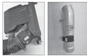
16. Remove the two screws securing the MAF sensor to the factory air box. Install the MAF sensor into the K&N<sup>®</sup> intake tube with the provided hardware.
