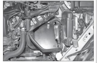
27. Install the heat shield into the engine bay, attach the side brackets to the vibration mount of the heat shield as shown.
