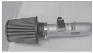
31. Install the K&N<sup>®</sup> air filter onto the intake tube as shown.
