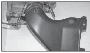
19. Unclip and remove the air inlet duct from the lower air box.
