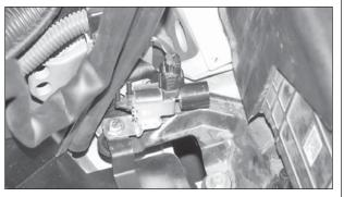
30. Reconnect the fresh air intake door vacuum switching valve solenoid electrical connection. NOTE: There will no longer be vacuum lines attached to the switching valve since the fresh air intake door has now been removed from the vehicle.
