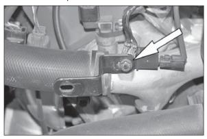
23. Install the "Z" bracket onto the ground with the provided hardware.
