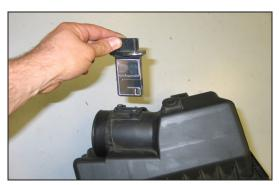
19. Remove the two screws securing the mass air sensor, and then remove the mass air sensor from the stock air box as shown.
