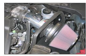
27. Install the K&N® air filter assembly onto the intake tube and secure with the provided hose clamp.
