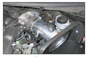
22. Install the K&N® intake tube into the silicone hose installed onto the throttle body and align it with the tube mounting bracket. Secure the intake tube with the hardware and hose clamp provided.
