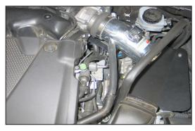
24. Install the crank case vent hose into the factory crank case vent hose and then connect the open end onto the K&N® intake tube as shown.
