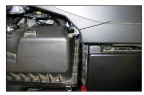
Remove the air box retaining bolt shown.
