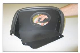
13. Install the provided edge trim into the hole of the heat shield as shown.
