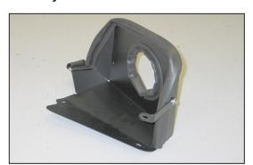
14. Install heat shield mounting bracket (070952) onto the heat shield as shown.
