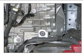
16. Install the longer rubber mounted stud onto the front air box mounting bracket as shown.
