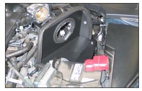
17. Install the heat shield assembly onto the rubber mounted studs installed in the previous steps and secure with the provided hardware. Secure the heat shield mounting bracket to the air box mounting bracket on the strut tower using the provided hardware.
