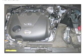
18. Re-install the fresh air intake duct onto the core support and into the heat shield and secure with the factory bolts.
