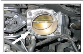
10. Remove the lower front throttle body mounting bolt shown. This bolt will be re-used in the next step.
