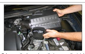
7. Loosen the hose clamp that secures the intake tube to the air box. Remove the stock air box from the vehicle.
