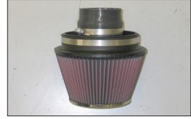
26. Install the K&N® air filter onto the air filter adapter assembly as shown.
