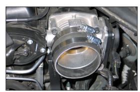
21. Install the silicone hose (08690) onto the throttle body and secure with the provided hose clamp.
