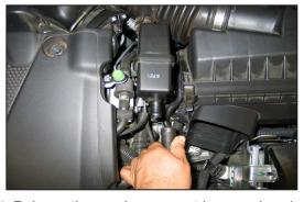
4. Release the crank case vent hose spring clamp and then disconnect the crank case vent hose from the intake tube resonator chamber.
