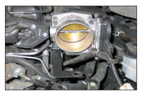
11. Using the bolt removed from the previous step, install the provided tube mounting bracket (070113) onto the throttle body as shown.
