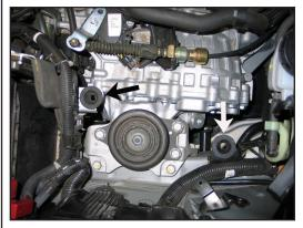
9. Remove the two rubber air box mounting grommets shown.
