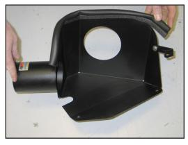
20. Install the provided edge trim onto the heat shield as shown.
