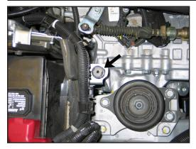
10. Install the 1.0" high rubber mounted stud onto the front air box mounting location using the provided hardware.
