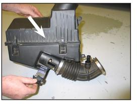
16. Remove the two bolts which secure the mass sensor to the intake tube and remove the mass air sensor as shown.
