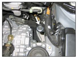
11. Install the ½" high rubber mounted stud onto the rear air box mounting location using the provided hardware.
