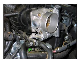
12. Remove the lower-front throttle body mounting bolt.NOTE: This bolt will be reused in the next step.
