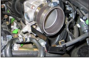
14. Install the provided silicone hose (084036) onto the throttle body and secure with the provided hose clamp.
