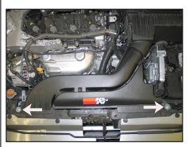
4. Remove the two bolts that secure the fresh air inlet assembly.
