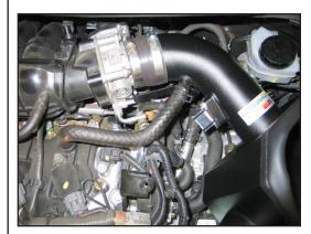
23. Install the factory crank case vent hose to the  $\frac{1}{4}$ " npt vent installed onto the K&N<sup>®</sup> intake tube.
