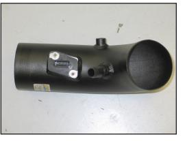
17. Install the mass air sensor into the K&N<sup>®</sup> intake tube and secure with the provided hardware.
