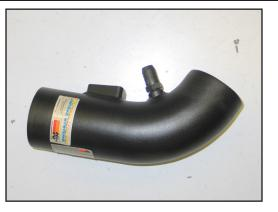
15. Install the provided  $\frac{1}{4}$  "npt vent fitting into the K&N® Intake Tube as shown.
