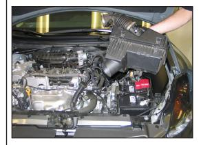
2. Disconnect the mass air sensor electrical connection and then unhook the wiring harness clips from the air box.
