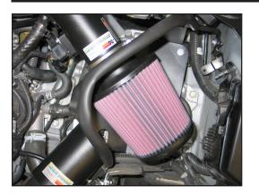
25. Install the K&N<sup>®</sup> air filter onto the K&N<sup>®</sup> intake tube and secure with the provided hose clamp. **NOTE: Drycharger<sup>®</sup> air filter wrap; part # RU-4990DK is available to purchase separately. To learn more about Drycharger<sup>®</sup> filter wraps or look up color availability please visit** http://www.knfilters.com<sup>®</sup>.
