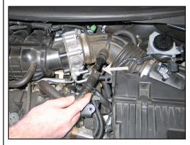
6. Release crank case vent hose spring clamp and then disconnect the crank case vent hose from the intake tube.
