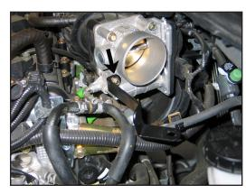
13. Install the tube mounting bracket (070091) onto the throttle body using the bolt removed in the previous step.
