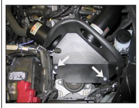
21. Install the heat shield into the vehicle so the mounting holes line up with the rubber mounted studs installed earlier. Secure the heat shield and mounting bracket with the hardware provided.
