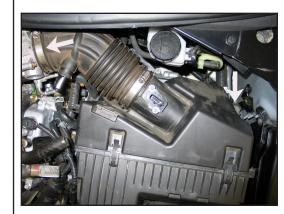
7. Loosen the hose clamp which secures the intake hose to the throttle body and remove the air box mounting bolt.
