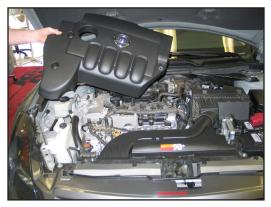
3. Remove three bolts which secure the engine cover and then remove the engine cover.
