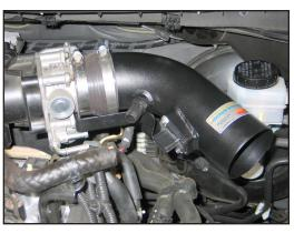
18. Install the K&N<sup>®</sup> intake tube into the silicone hose at the throttle body and align with the mounting bracket. Secure with the provided hardware and hose clamp.
