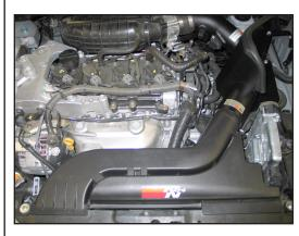
22. Reinstall the fresh air inlet supply to the original location and into the fresh air tube on the heat shield then secure with the factory bolts.
