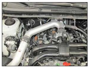
21. Install the remaining coupling hose onto the intake tube and Install the intake tube into the hoses and adjust the tubes for best fit. Then secure the provided hose clamps.
