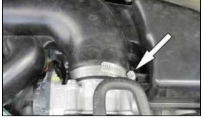
4. Loosen the hose clamp securing the intake tube to the throttle body.
