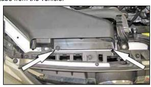
6. Remove the two plastic clips securing the intake scoop to the core support and then remove the intake scoop from the vehicle.
