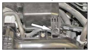
3. Remove the plastic clip which secures the intake plenum to the intake manifold.
