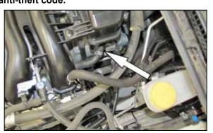
2. Release the spring clamp securing the crank case vent hose to the intake plenum and then disconnect the hose from the plenum.
