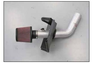
16. Install the K&N® air filter onto the intake tube and secure with the provided hose clamp.
