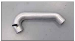
19. Install the 90° NPT vent fitting into the K&N $^{\! \rm 8}$  intake tube as shown.
