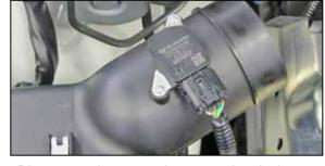
7. Disconnect the mass air sensor electrical connection.
