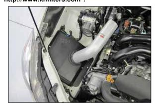
17. Install the intake tube/heat shield assembly into the engine compartment as shown and secure with the provided hardware and factory nuts from step 8. NOTE: Install the heat shield onto the factory studs first and then align the bottom hole for the bolt.
