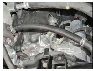
23. Install the open end of the hose mender into the factory crank case vent hose and then connect the hose to the fitting installed into the K&N® intake tube.
