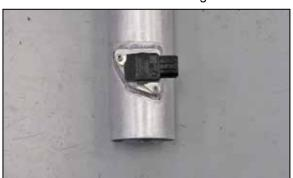
13. Install the mass air sensor into the K&N® intake tube and secure with the provided hardware.
