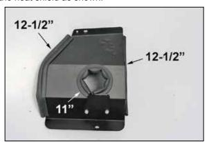
11. Cut the provided edge trim into three sections, two sections should be 12-1/2" long and one section should be 11" long. Install the edge trim onto the heat shield as shown.
