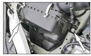
8. Remove the bolt and nut that secure the air filter housing into the vehicle and then remove the air filter housing from the vehicle.
