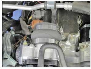
18. Install one of the provided coupler hoses onto the throttle body and secure with the provided hose clamp.
