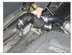
9. Remove the stock intake tube from the vehicle. NOTE: K&N Engineering, Inc., recommends that customers do not discard factory air intake.
