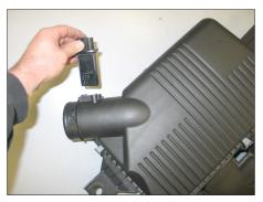
15. Remove the mounting screws and then remove the mass air sensor from the stock air box.
