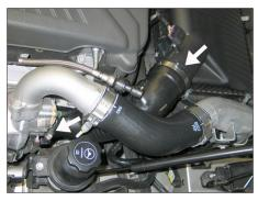
4. Loosen the hose clamps which secure the intake tube to the turbo inlet and air box.
