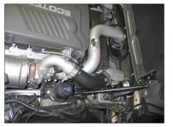
10 Install the K&N® intake tube into the silicons
