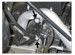
6. Remove the two bolts which secure the left side intercooler tube mounting bracket and then remove the bracket.
