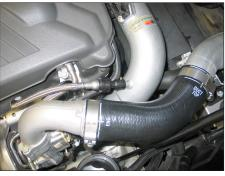
20. Connect the crank case vent fitting to the fitting on the K&N $^{\mbox{\tiny B}}$  intake tube.
