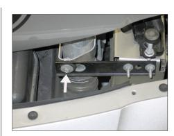
7. Remove the bolt which secures the left side intercooler tube to the front mounting bracket. **NOTE: This bolt will be reused.**
