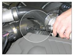
3. Release the crank case vent line retaining clip and then disconnect the crank case vent line.
