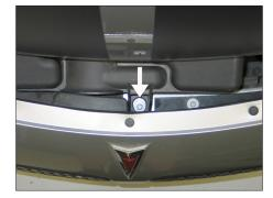
5. Remove the bolt which secures the front of the
