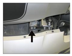
10. Reinstall the bolt which secures the left side intercooler tube to the front mounting bracket.
