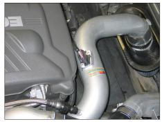
21. Reconnect the mass air sensor electrical connection.
